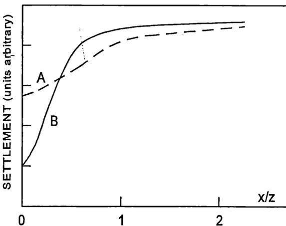
Fig. 2b. Computed settlement troughs
