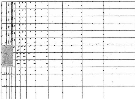
Fig. 2a. Rough finite element model of tunnel.
