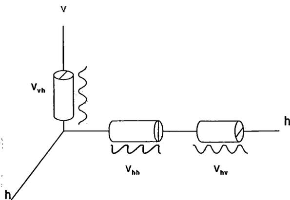
Fig. 3. Shear waves in laboratory samples
