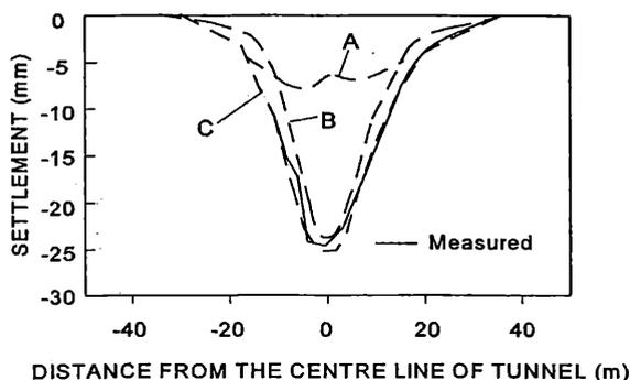
Fig. 6. Computed settlement troughs for trial tunnel
