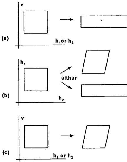
Fig. 1. Modes of shear deformation
