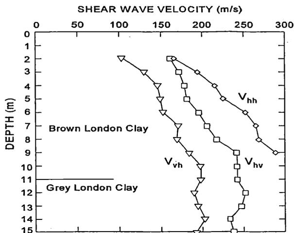
Fig. 5. In situ shear wave tests in London Clay
