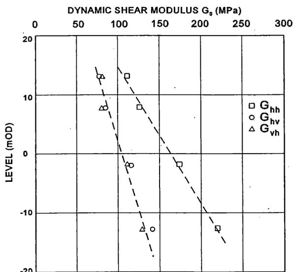
Fig. 4.  $G_0$  measured in bender element tests
