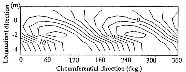
Fig. 6. (a) Distribution of normal displacement of ground (mm)
