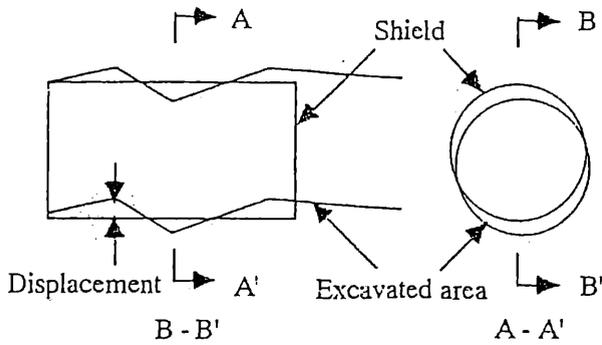
Fig. 3. Displacement and excavated area
