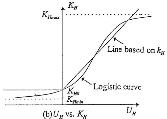
Fig. 2. Displacement vs. coefficient of earth pressure
