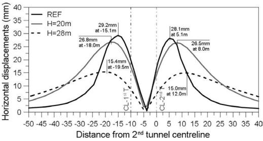
Figure 14. Influence of the depth of the tunnel on the horizontal displacements (absolute values).
