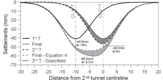
Figure 6. Settlement troughs obtained in the reference analysis.
