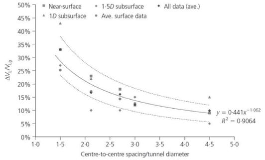
Figure 3. Increases in the second tunnel volume loss in comparison with first tunnel (after Divall (2013)).
