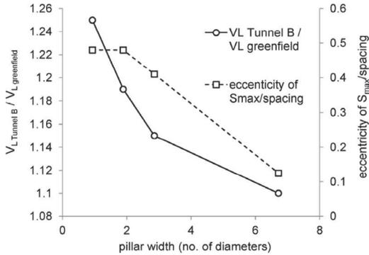
Figure 2. Addenbrooke & Potts (2001) proposal for determine the volume loss (left) and eccentricity of the maximum settlement (right) of the second tunnel excavated (Tunnel B).
