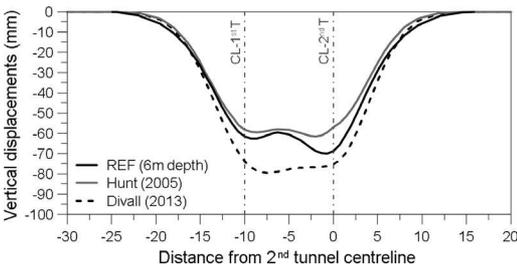
Figure 9. Final sub-surface vertical displacements at 6 m depth estimated by the proposed methods.
