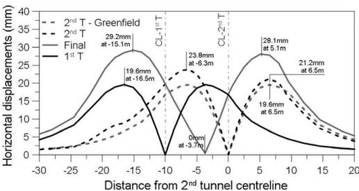
Figure 10. Horizontal displacements obtained for the reference analysis (absolute values).
