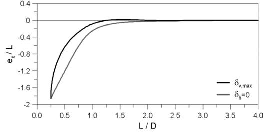
Figure 19. Influence of the pillar width on the eccentricity of the final displacements.
