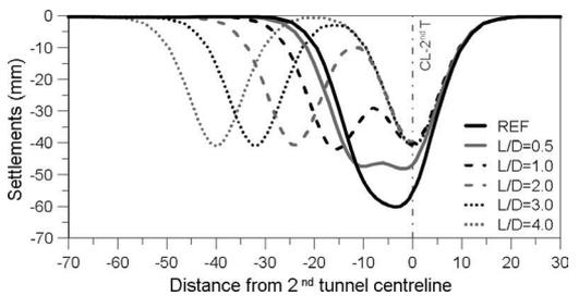
Figure 16. Influence of the pillar width on the settlement troughs.
