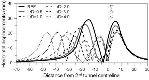
Figure 17. Influence of the pillar width on the horizontal displacements (absolute values).
