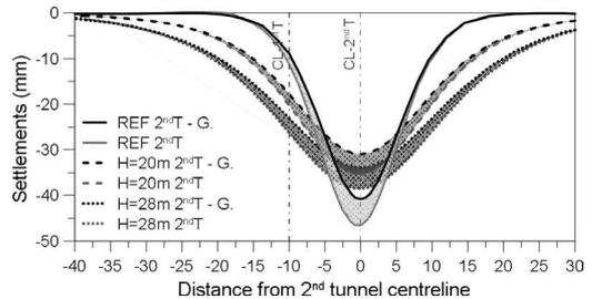
Figure 13. Settlement troughs induced by the excavation of the 2nd Tunnel for different depths.
