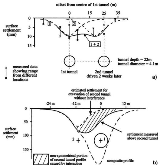
Figure 1. Settlements induced by the excavation of twin tunnels: a) Bartlett & Bubbers (1970); b) Cording & Hansmire (1975).
