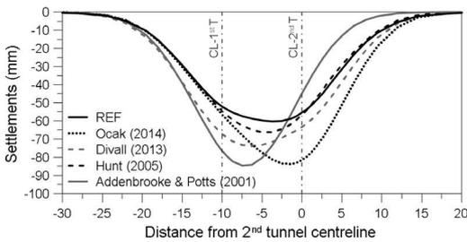
Figure 7. Final settlement troughs estimated by the proposed methods.
