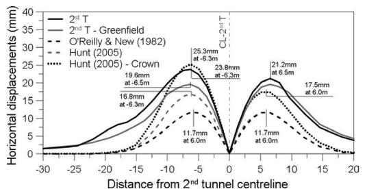
Figure 11. 2nd Tunnel horizontal displacements estimated by the proposed methods (absolute values).
