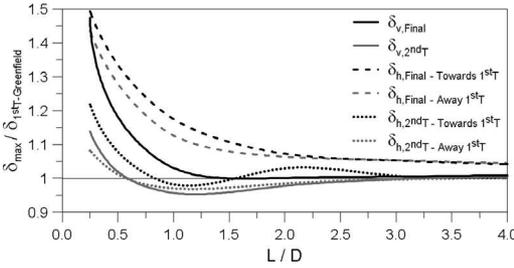
Figure 18. Influence of the pillar width on the maximum vertical and horizontal displacements.
