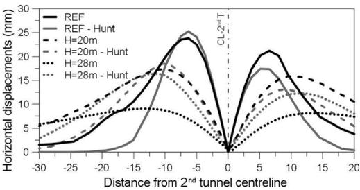
Figure 15. Influence of the depth of the tunnel on the 2nd Tunnel horizontal displacements (absolute values).
