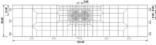
Figure 5. Reference finite element mesh.
