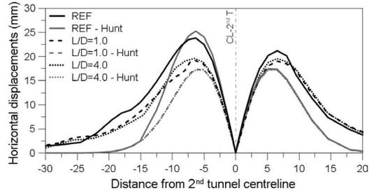
Figure 20. Influence of the pillar width on the 2nd Tunnel horizontal displacements (absolute values).
