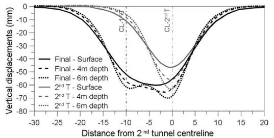
Figure 8. Final sub-surface vertical displacements at different depths.
