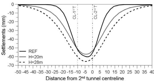
Figure 12. Influence of the depth of the tunnel on the settlement troughs.
