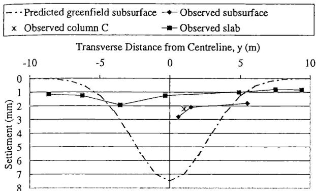
Figure 4. Predicted ( $V_L = 0.8\%$ ) and measured transverse settlements.
