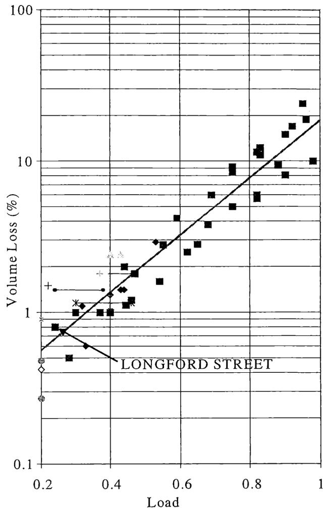
Figure 3. Volume loss – load factor relationship.
