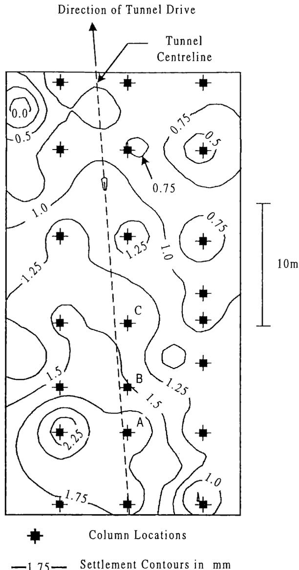
Figure 5. Contour plot of slab settlements, 26<sup>th</sup> August 1997.
