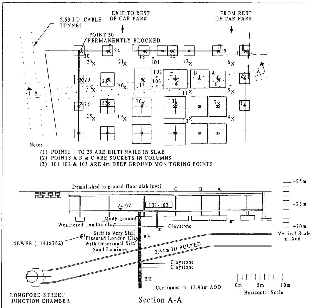
Figure 2. Plan and section through site showing monitoring layout.
