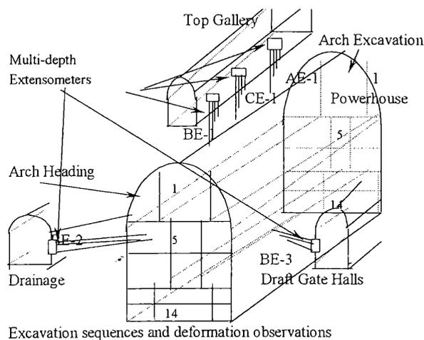
Figure 2. Excavation stages for powerhouse caverns.
