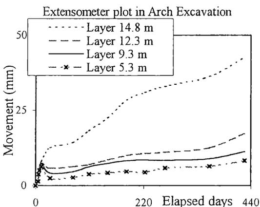
Figure 3. Deformations at sta. 0+51.5 from (BE-1).
