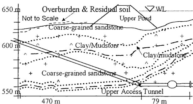
Figure 1. Sketch of upper access tunnel to penstock.
