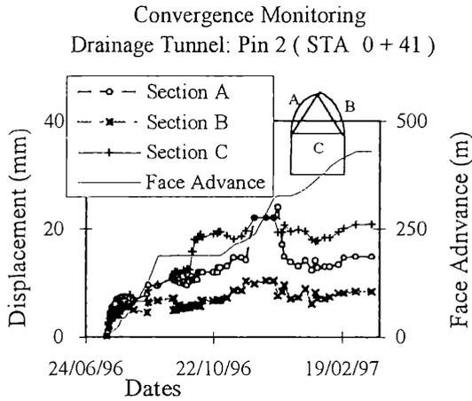
Figure 5. Deformation plot in drainage tunnel at sta. 0+41 m.
