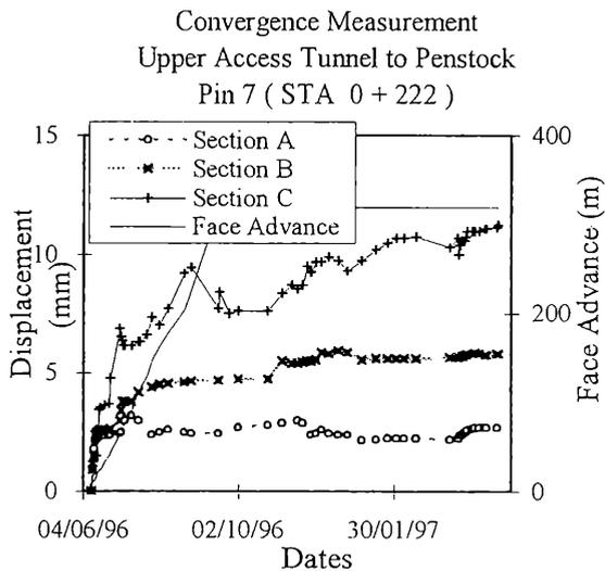
Figure 6. Deformation plot in upper access tunnel to penstock at sta. 0+222 m.
