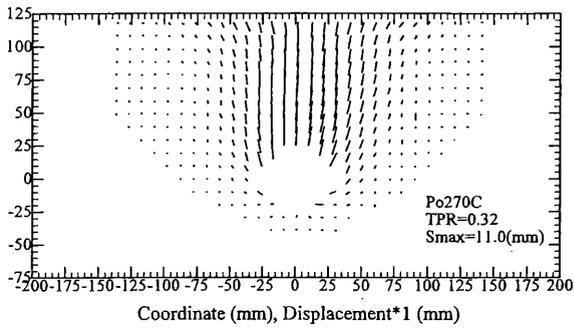
Figure 7. Deformations in the model of Po270C.
