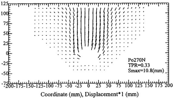
Figure 8. Deformations in the model of Po270N.
