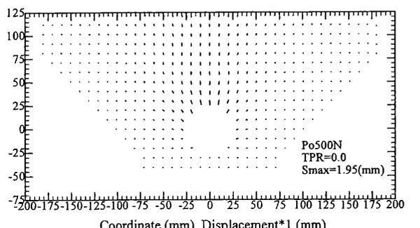
Figure 12. Deformations in the model of Po500N.
