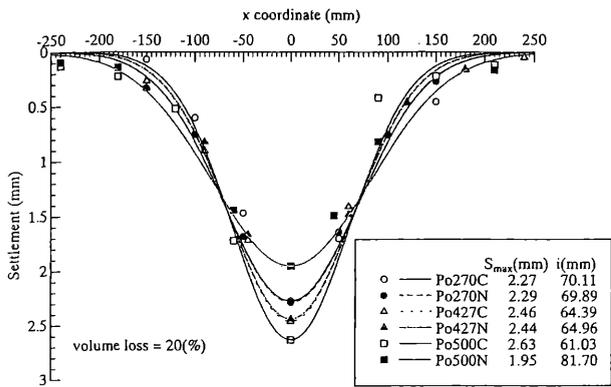
Figure 4. Settlement troughs at the ground surface.
