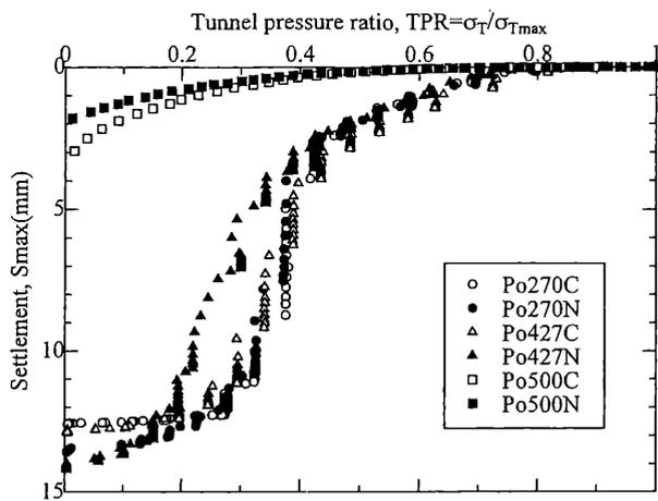
Figure 3. Settlements with the reduction in the tunnel support pressure.
