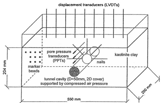
Figure 1. Schematic diagram of centrifuge model.
