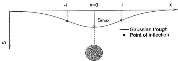
Figure 5. Approximation of settlement trough by Gaussian distribution.
