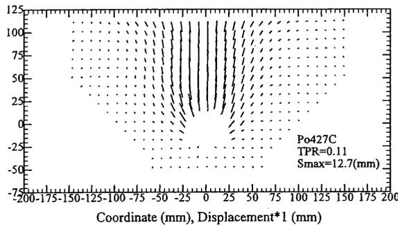
Figure 9. Deformations in the model of Po427C.
