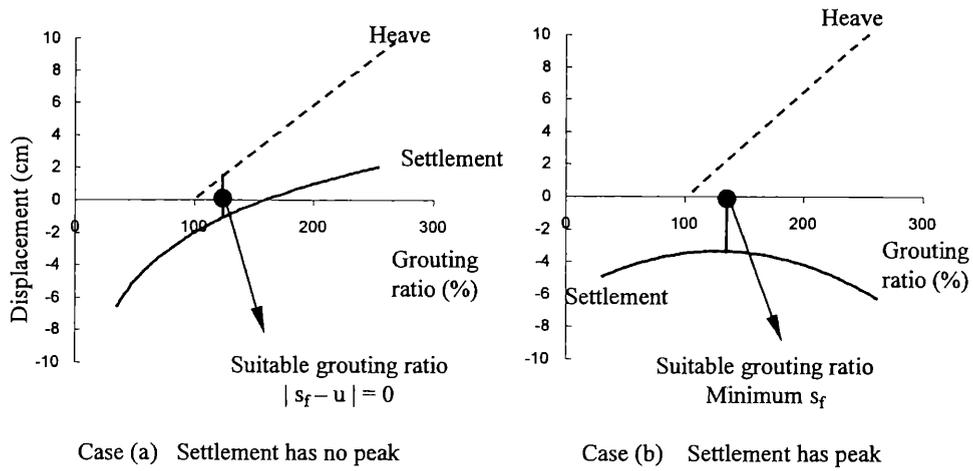
Figure 7 Determination of suitable grouting ratio.
