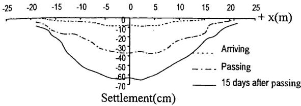
Figure 9 Transverse surface settlement trough.
