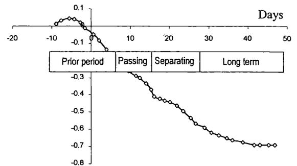
Figure 8 Ground surface deformation above the tunnel axis.
