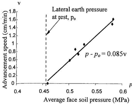
Figure 5 Relationship between advancement speed and face earth pressure.
