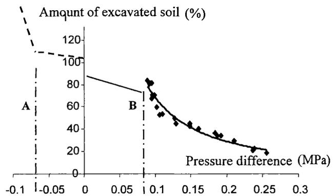
Figure 4 Relationship of amount of excavated soil and pressure difference.
