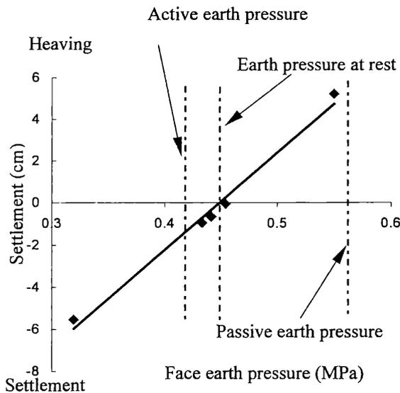
Figure 3 Relationship between face pressure and ground surface settlement.
