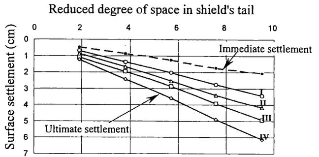
Figure 6 Relationship between ground surface settlement vs. the time to start grouting.
