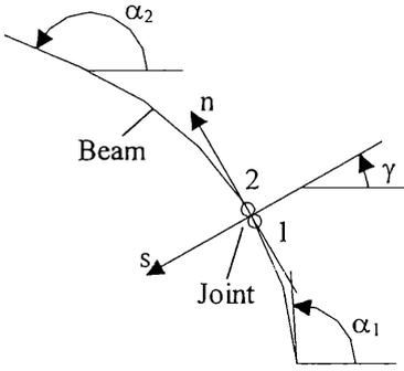
Figure 1. Curved beam-joint model.
