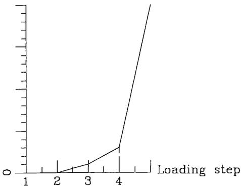
Figure 5. The maximum normal stress  $\sigma_n$  of the contact element versus the loading step.
