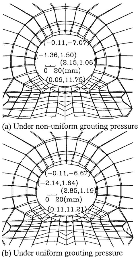
Figure 7. The displaced mesh in loading step No.4
