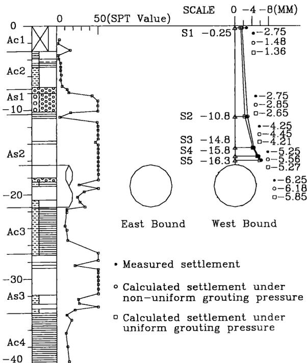
Figure 3. The soil layers of B section and the measured/calculated settlements above the tunnel.
