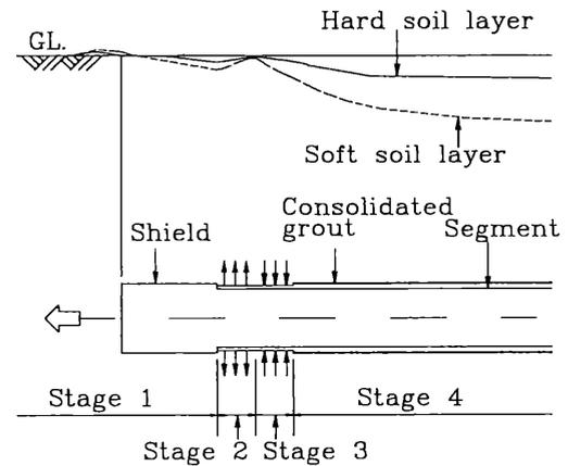
Figure 2. Diagram of the construction process of shield tunneling.
