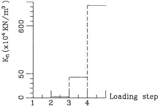
Figure 4. The normal stiffness  $K_n$  of the contact element versus the loading step.
