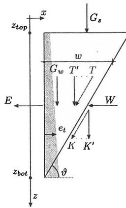
Figure 2. Definition of forces acting on the wedge and infiltration zone (shaded area).
