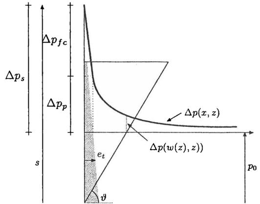
Figure 3. Pressure drop over penetration zone and excess pore pressure distribution.
