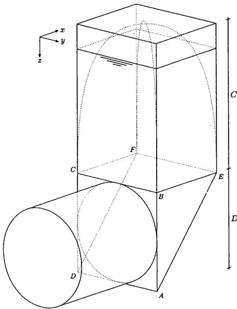
Figure 1. Wedge and silo model.
