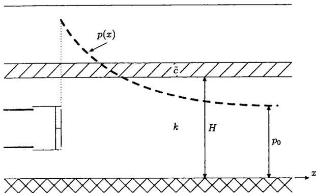
Figure 4. Schematisation of semi-confined aquifer.
