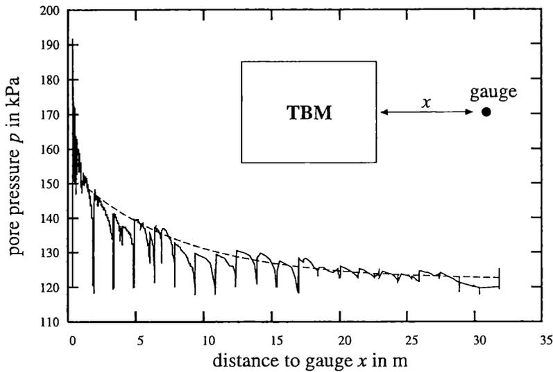
Figure 5. Excess pore pressure measurements taken at the Second Heineoord Test Field North, adapted from Bezuijen (1998), compared to calculated pore pressure distribution (dashed line).
