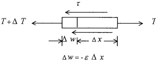
Figure 2. Free body diagram for bolt element.
