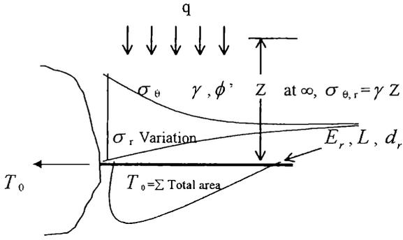
Figure 1. Underground stresses around rock-bolt.
