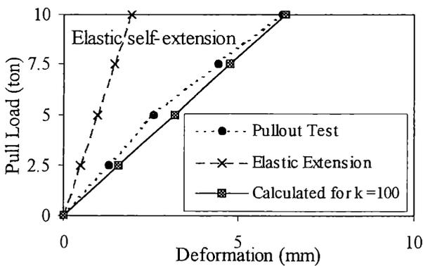
Figure 4. Rock-bolt pullout deformations at sat. 0+100 m in upper access tunnel to penstock.
