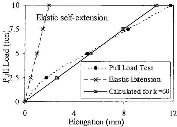
Figure 3. Rock-bolt pullout deformations at sta. 0+74 m in top gallery.
