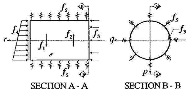
Figure 1. Model of loads acting on shield.
