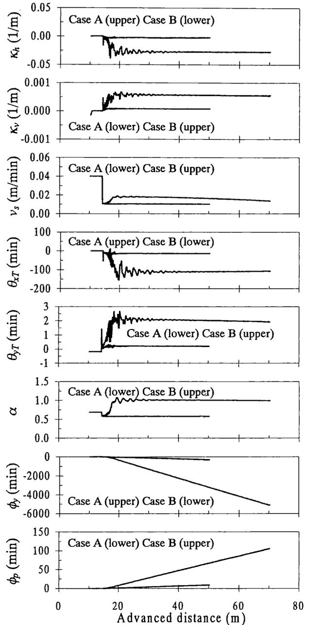
Figure 5. Parameters during shield behaviour simulation.
