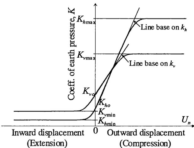
Figure 2. Ground reaction curve for  $K_h$  and  $K_v$ .
