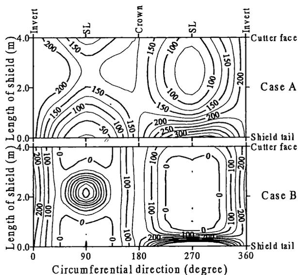
Figure 7. Effective normal earth pressure around the shield ( $\text{kN/m}^2$ ).
