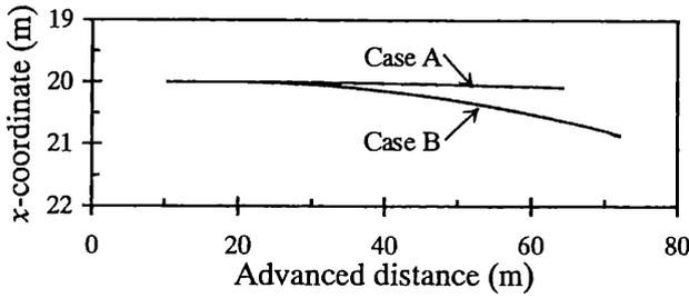
Figure 4(a). Trace of shield in vertical plane.
