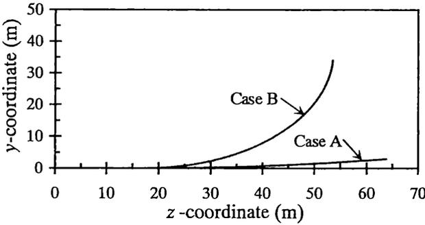
Figure 4(b). Trace of shield in horizontal plane.
