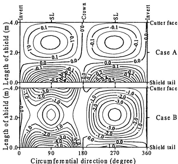
Figure 6. Normal ground displacement around the shield (cm).
