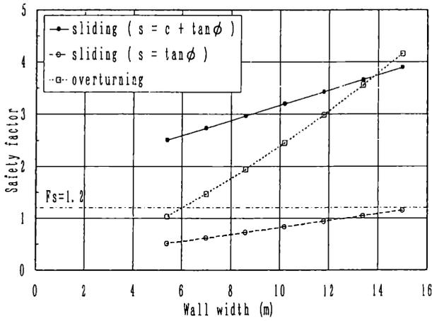
Figure 9. Relationship between the sliding and overturning safety factor ( $F_s$ ) and the wall width
