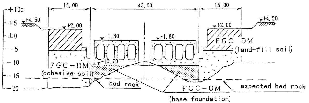
Figure 1. Standard section of pump pit.
