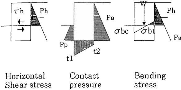
Figure 7. Design Method (simplified processes)
