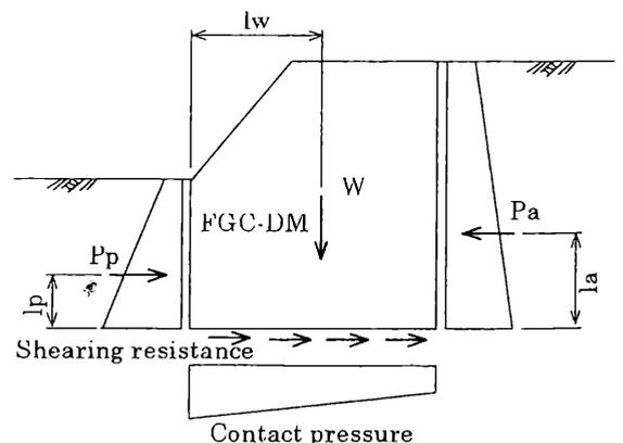
Figure 6. Application of external force
