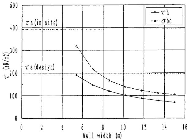
Figure 10. The relationship between the shear stress and wall width.
