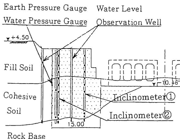
Figure 3. The earth retaining cross section
