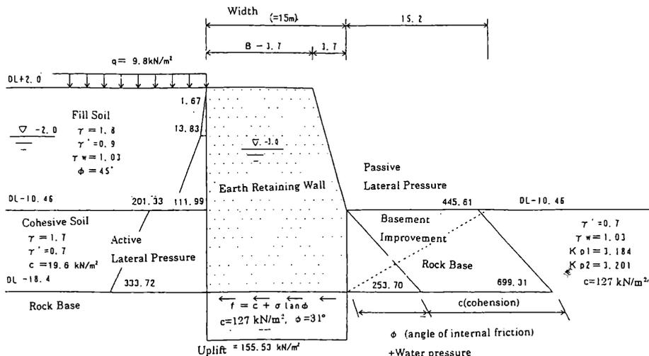
Figure 8. The lateral earth pressure and uplift on the wall
