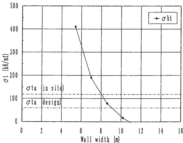
Figure 11. The relationship between the tensile stress and wall width.
