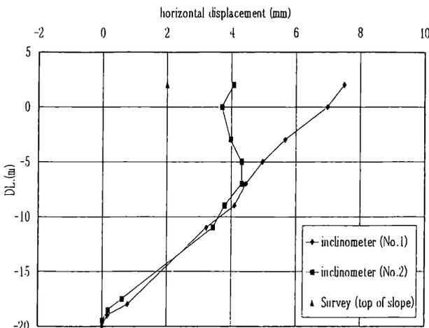
Figure 5. The depth distribution of the displacement
