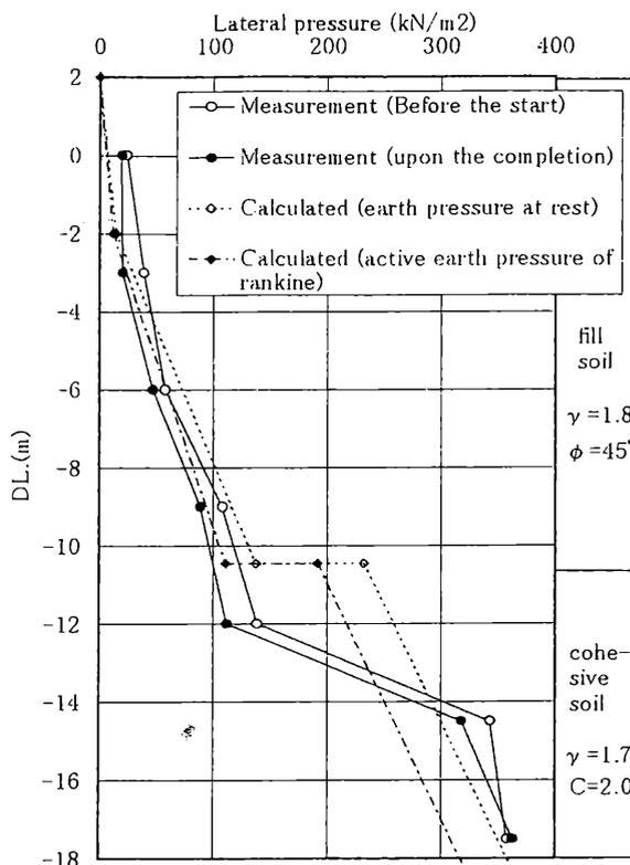
Figure 4. The lateral pressure exerted the back side of the wall
