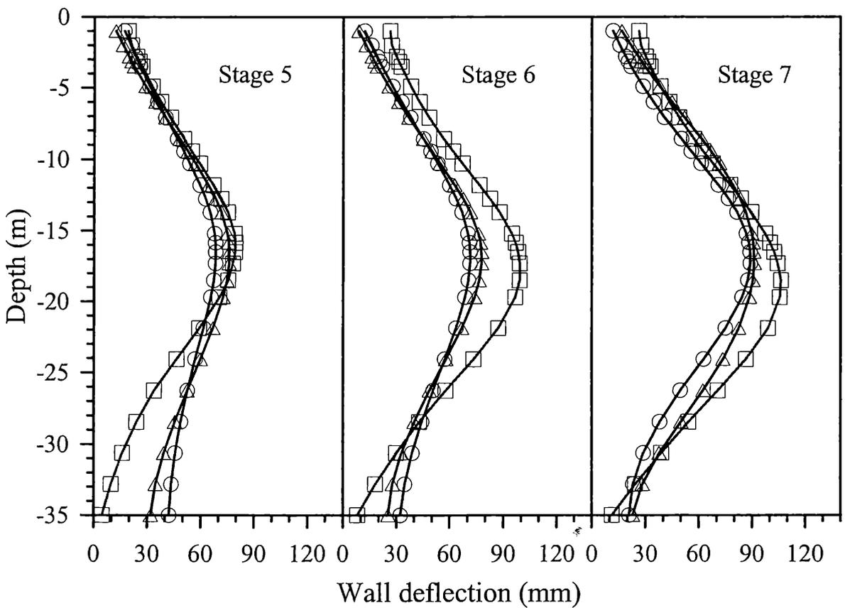
Figure 4. Wall deflection profiles in various excavation stages.
