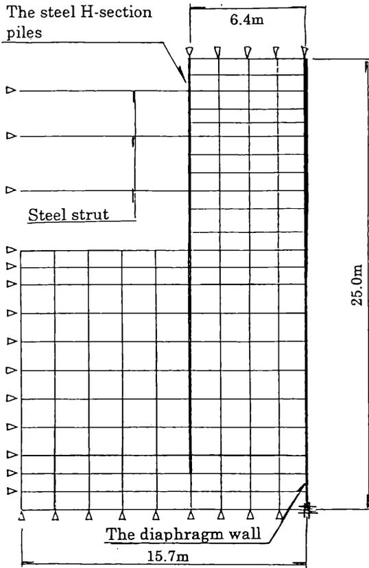
Figure 9. Finite Element Method model for the 10<sup>th</sup> excavation step.
