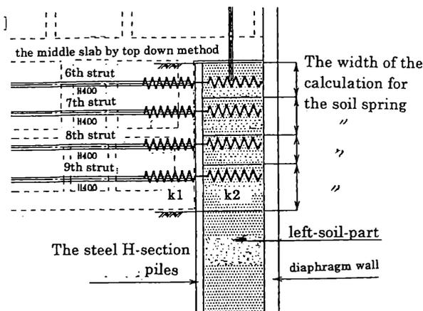
Figure 7. The series linear spring of the original design.
