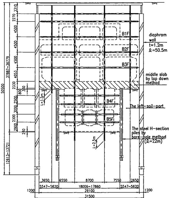
Figure 4. The typical cross section of the excavation.
