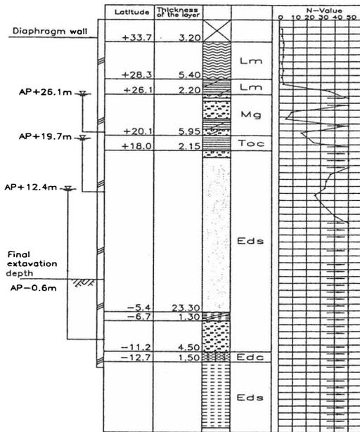
Figure 3. Soil profile at the excavation site.
