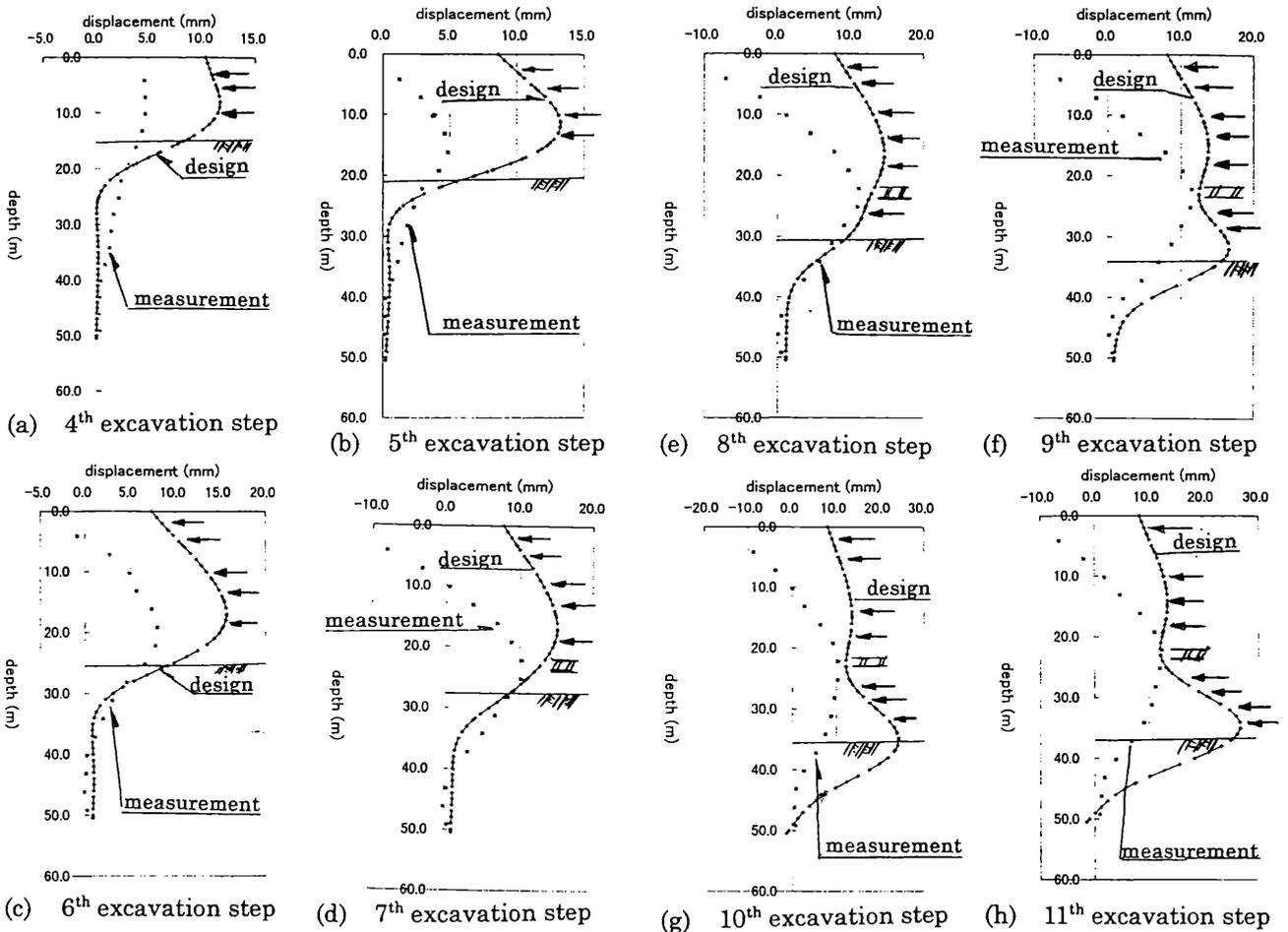
Figure 6. Comparison about the displacement of diaphragm wall at 4<sup>th</sup> -11<sup>th</sup> excavation step
