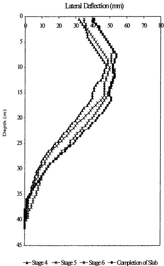
Figure 4. Measured lateral wall displacement.
