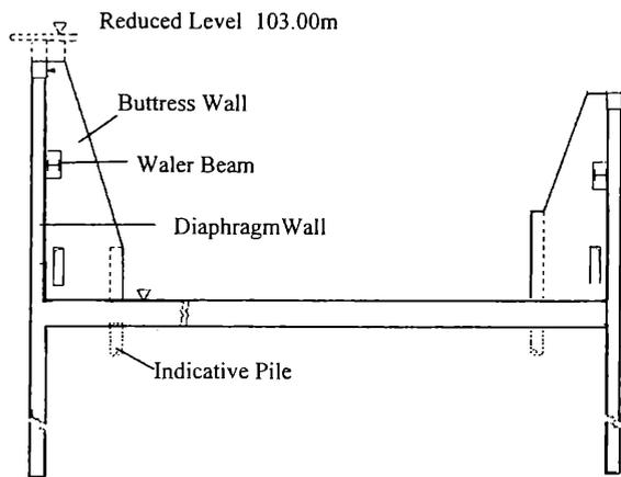
Figure 3. Typical section view of buttress walls.
