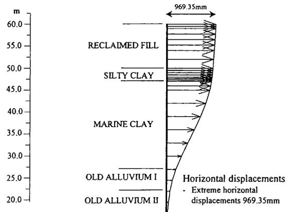
Figure 6. Computed deformation profile of diaphragm wall.
