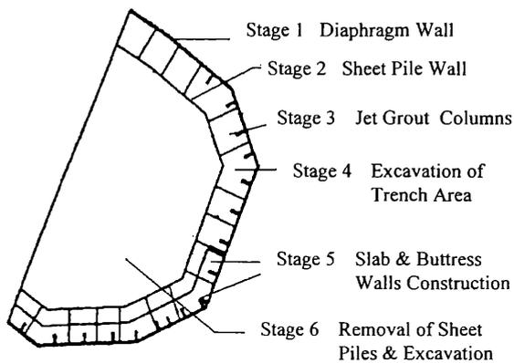
Figure 2. Construction and excavation sequence.
