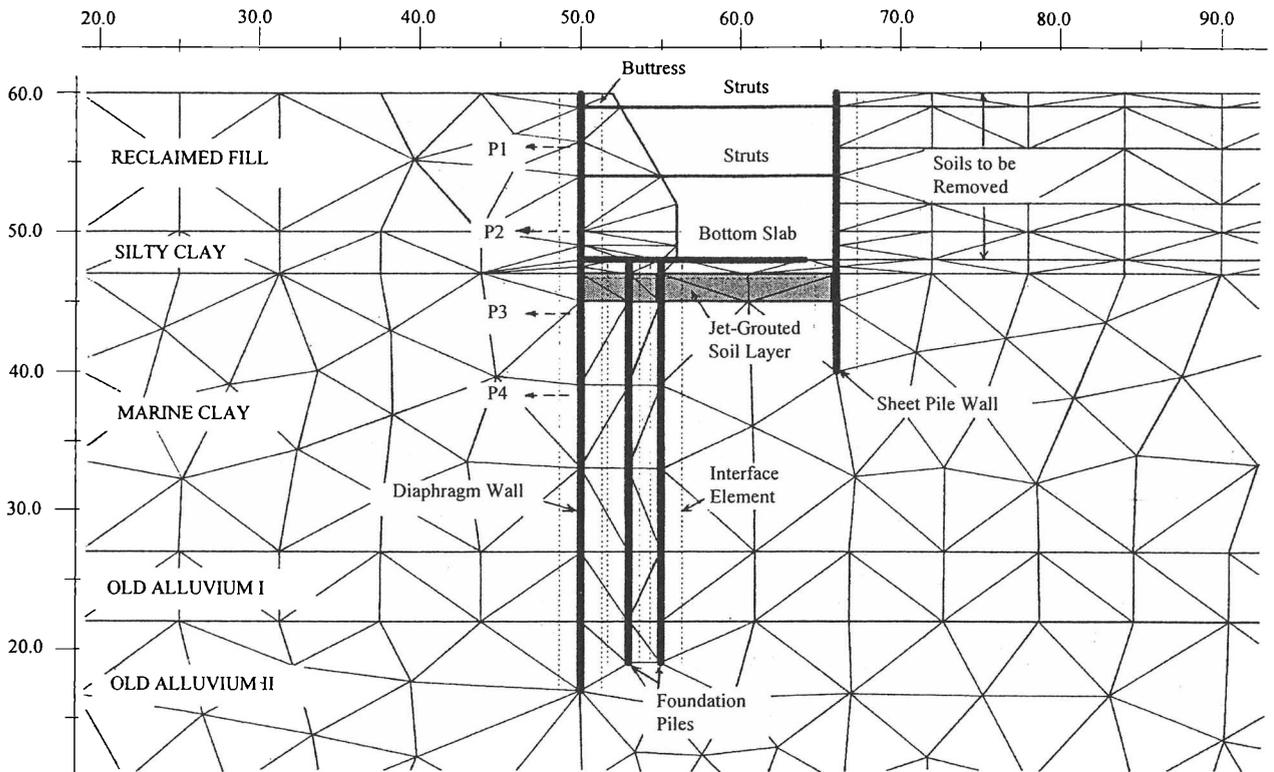
Figure 5. Close-up view of finite element mesh (Refer to Stage 5 of Figure 2).
