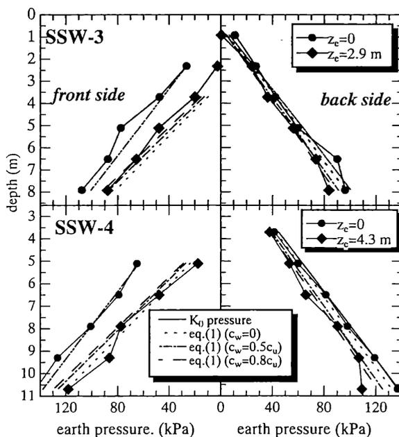
Figure 11. Total earth pressure on the wall surface.
