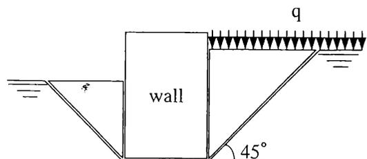
Figure 10. Failure mechanism used in the upper bound analysis.
