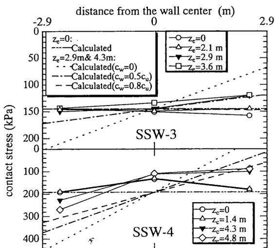
Figure 12. Contact pressures at wall base.
