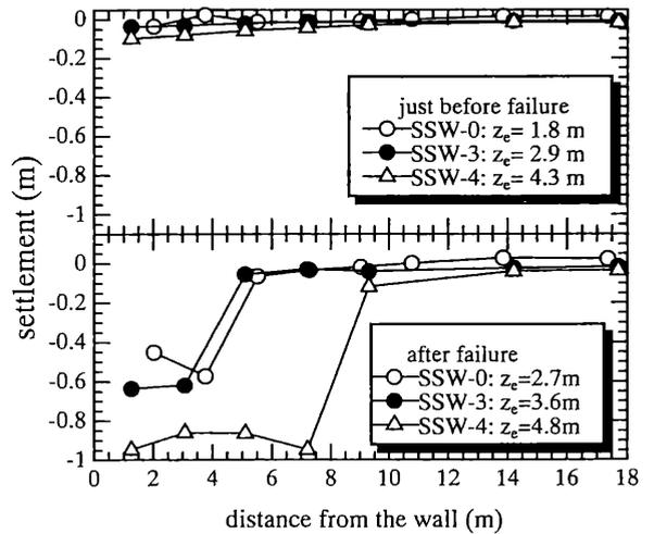
Figure 9. Settlement distribution behind the wall.
