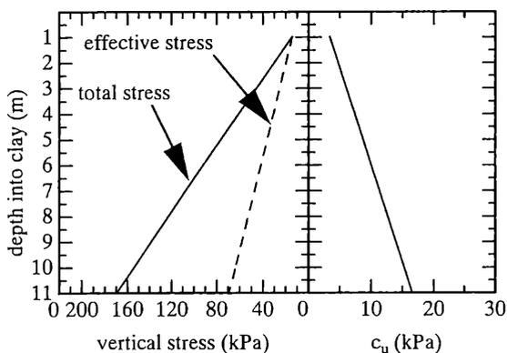
Figure 4. Profile of vertical stress and undrained compressive strength in clay.
