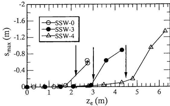
Figure 7. Variation of max. settlement behind the wall
