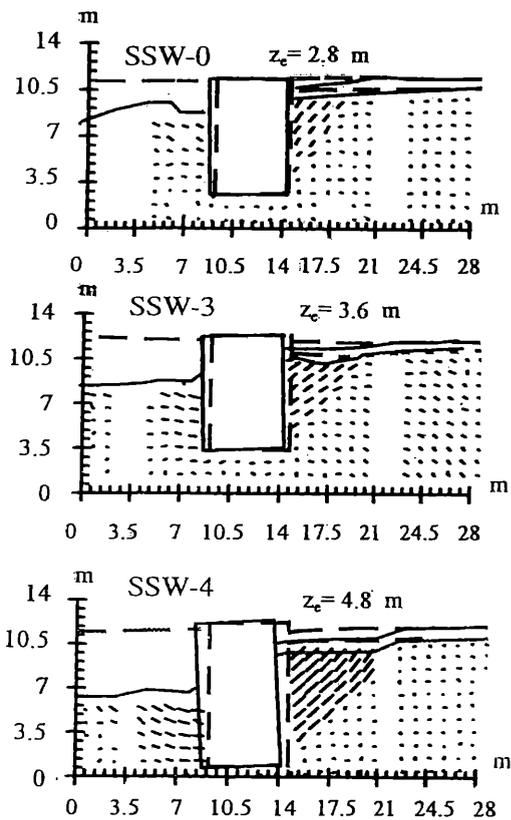
Figure 8. Observed deformation in the ground.
