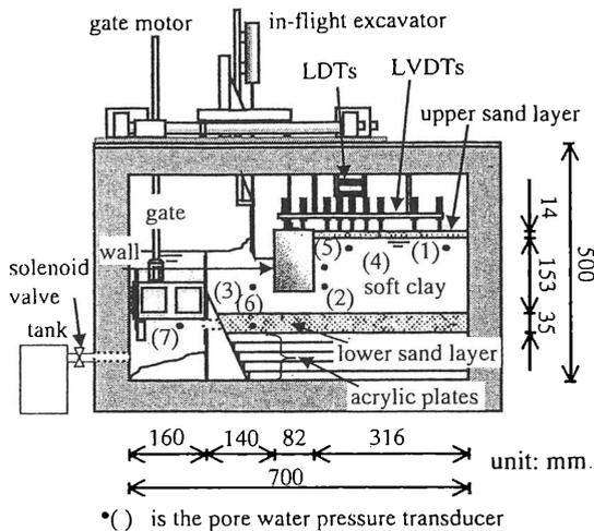
Figure 1. Test setup.
