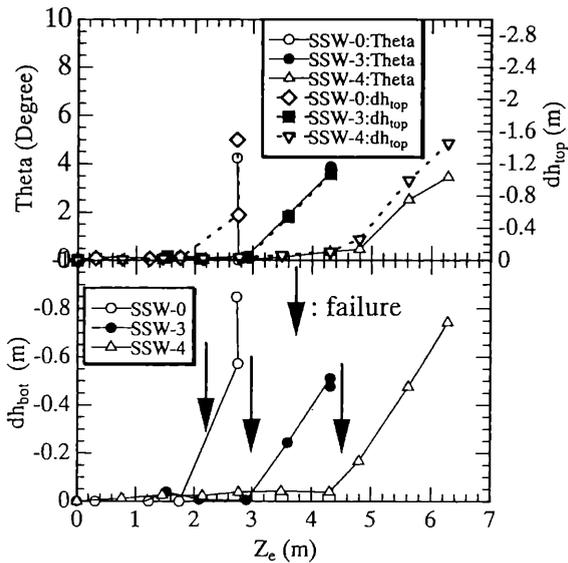
Figure 6. Variation of horizontal top and bottom displacements and tilting of wall during excavation.
