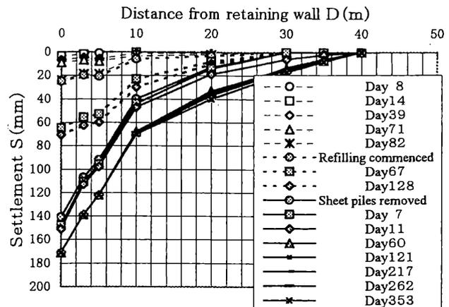
Figure 4(a). Variation of settlement with distance (at Section C).
