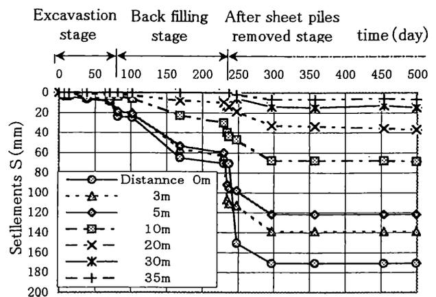
Figure 4(b). Progress of settlement with time (at Section C).
