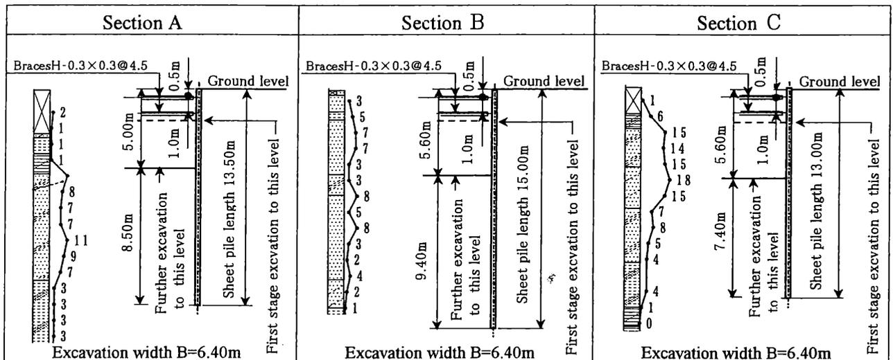
Figure 2. Details of the works at three sections.
