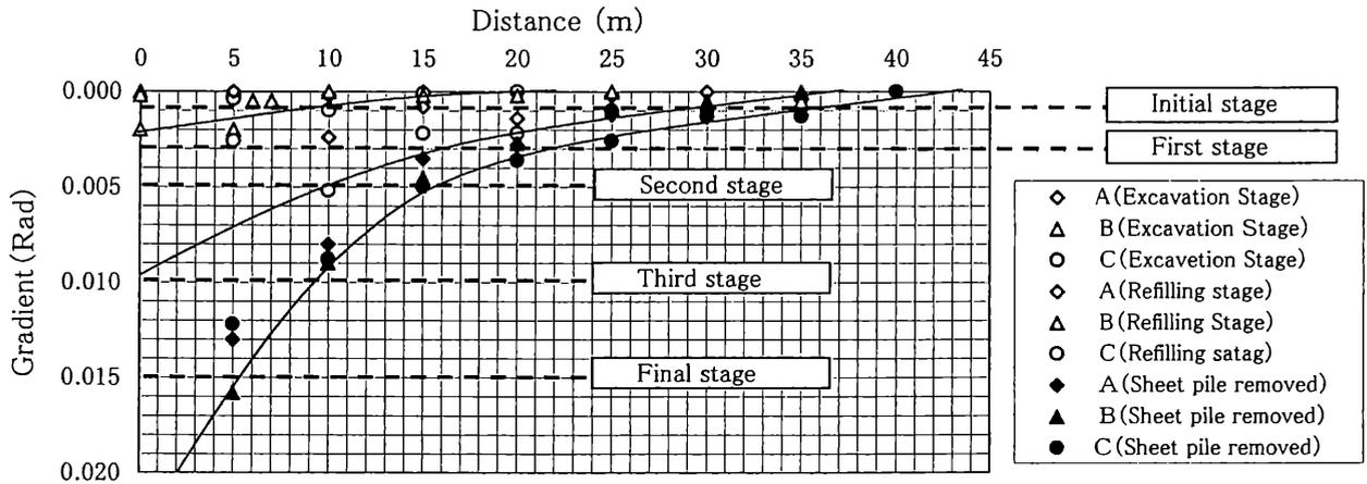
Figure 7 . Variation in Gradient with Distance Various Stage of work.
