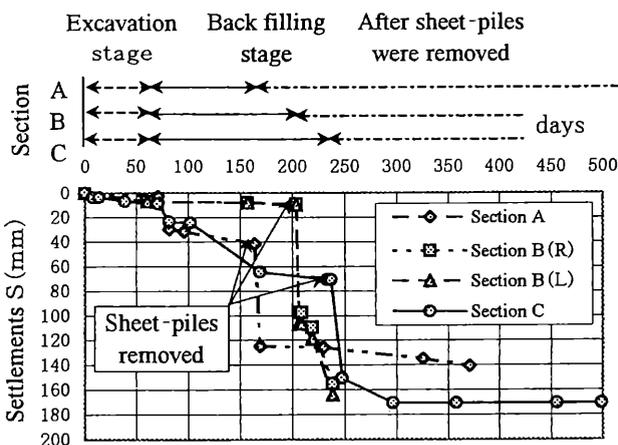
Figure 5. Progress of settlement with time.
