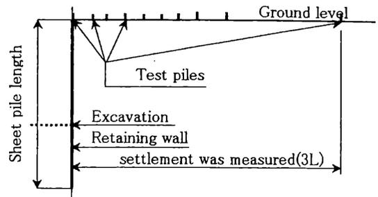
Figure 3. Test pile arrangement.
