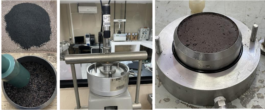
Figure 3: Soil mixture, specimen compaction, and oedometer equipment.
