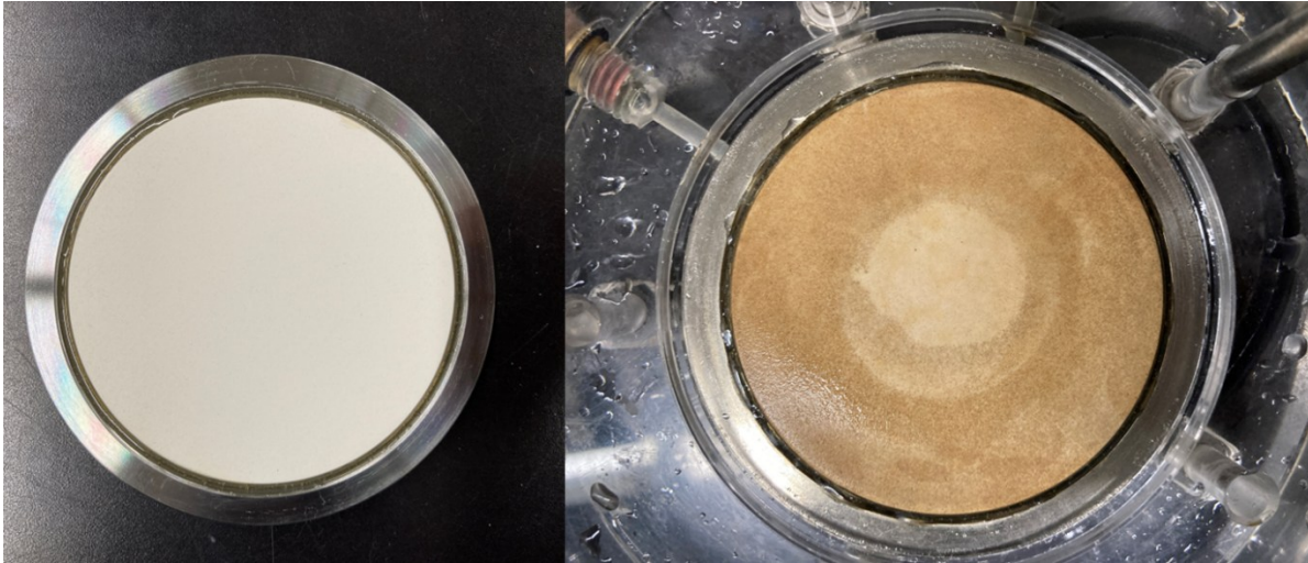
Figure 2: Comparison between a new (left) and a used, bitumen-stained (right) ceramic plate.
