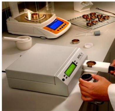
Figure 8: High soil suction range Chilled-Mirror PotentiaMeter for measuring the w -SWCC relationship [15].
