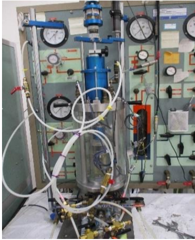
Figure 1: Developed cyclic triaxial test apparatus.
