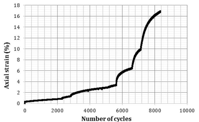
Figure 10. Liquefaction of unsaturated samples axial strain versus number of cycle.
