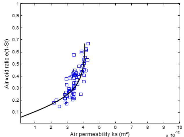
Figure 3. Air permeability tests results for Fontainebleau sand.
