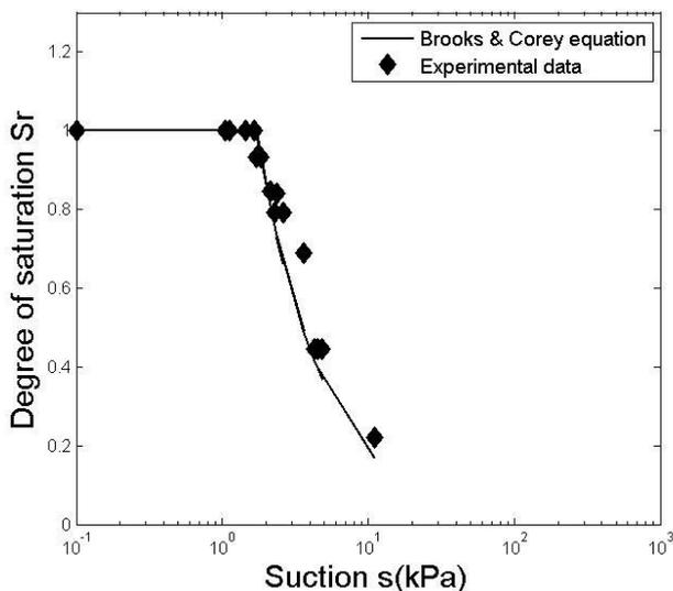
Figure 1. Soil-water characteristic curve – Experimental and model.
