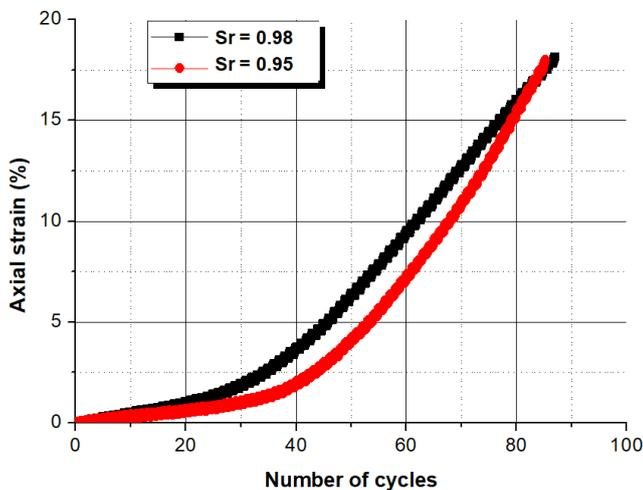
Figure 8. Liquefaction of nearly saturated samples axial strain versus number of cycle.
