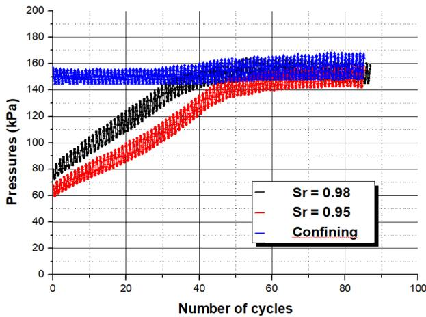
Figure 7. Liquefaction of nearly saturated samples water pressure versus number of cycle.
