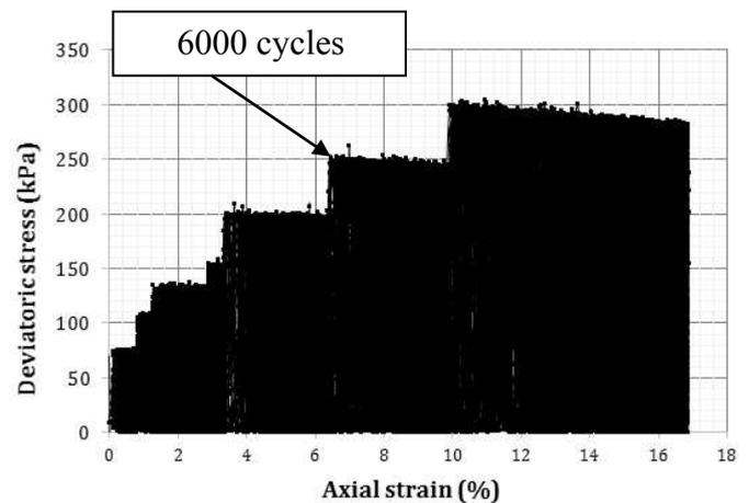
Figure 9. Liquefaction of unsaturated samples deviatoric stress versus axial strain.
