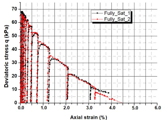
Figure 6. Liquefaction of saturated samples deviatoric stress versus axial strain.
