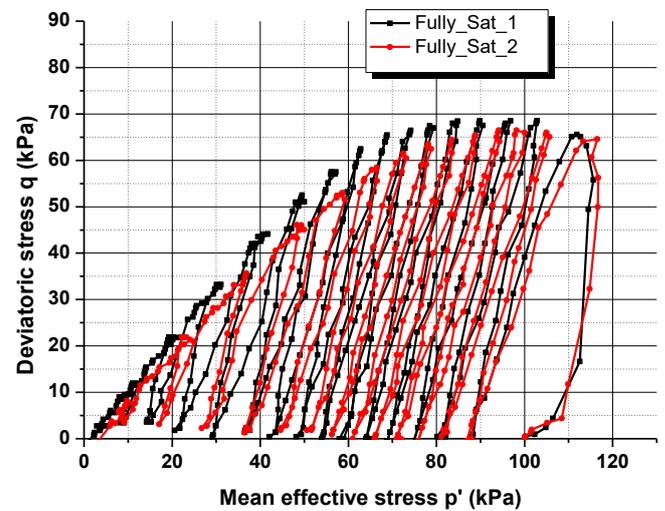
Figure 5. Liquefaction of saturated samples deviatoric stress versus mean effective stress.
