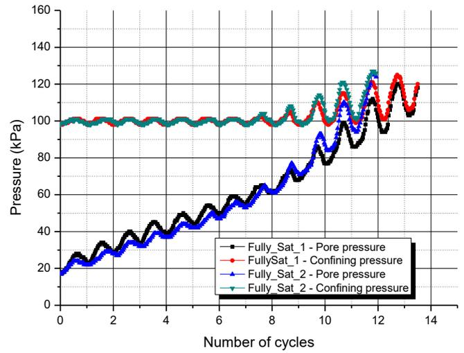
Figure 4. Liquefaction of saturated samples water pressure versus number of cycle.
