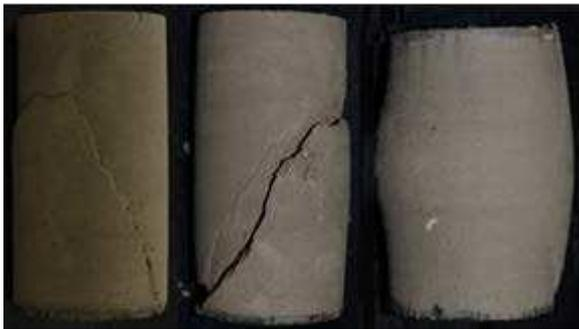
Figure 3. Soil specimens after the triaxial test.
