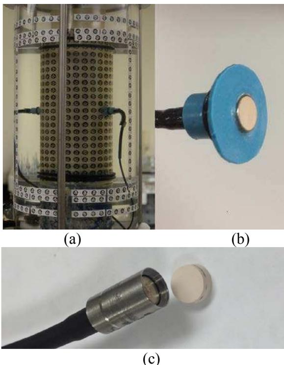
Figure 1. Triaxial testing system and high-capacity tensiometer.
