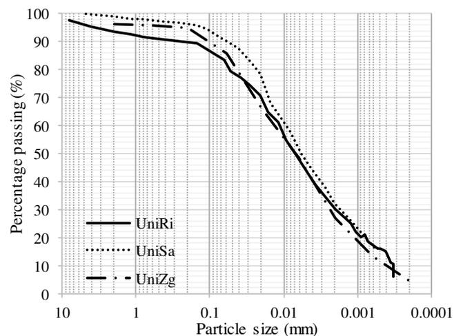
Figure 1. Grain size distribution test results.
