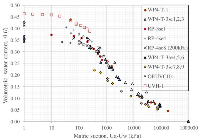
Figure 5. Results obtained using different devices and techniques for SWRCs determination.
