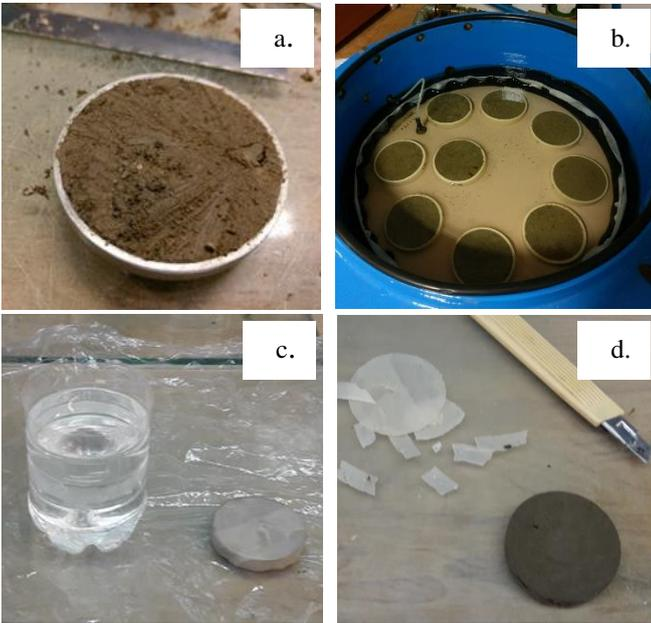
Figure 2. Some details of specimen preparation for RP-3 test (a: soil sample, b: saturation inside the pressure plate extractor device, c: specimen coated in wax, d: wax removal after measurements).
