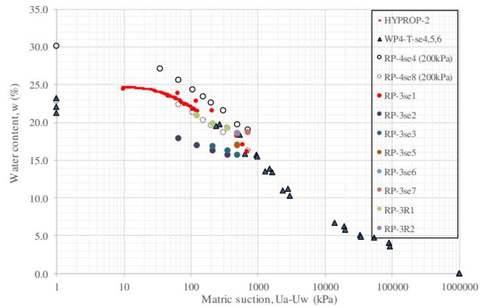
Figure 3. Results for RP-3 and RP-4 test with results obtained using WP4-T and HYPROP devices in drying process.
