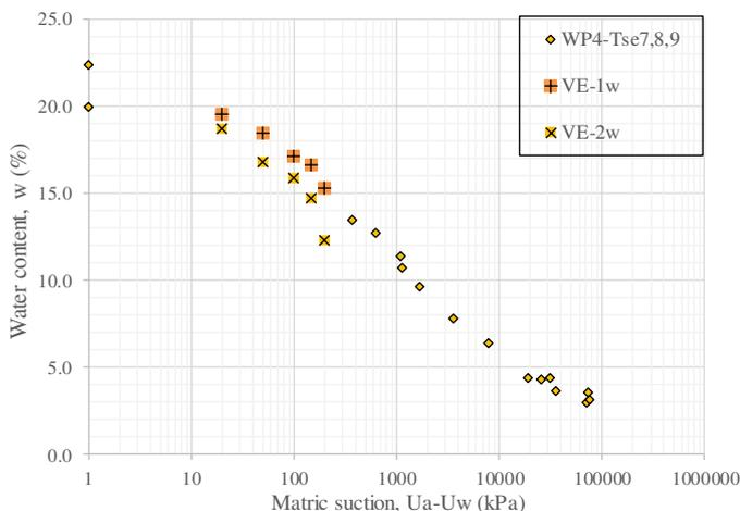
Figure 4. Results from VE1w and VE2w tests with results obtained using WP4-T device in wetting process.
