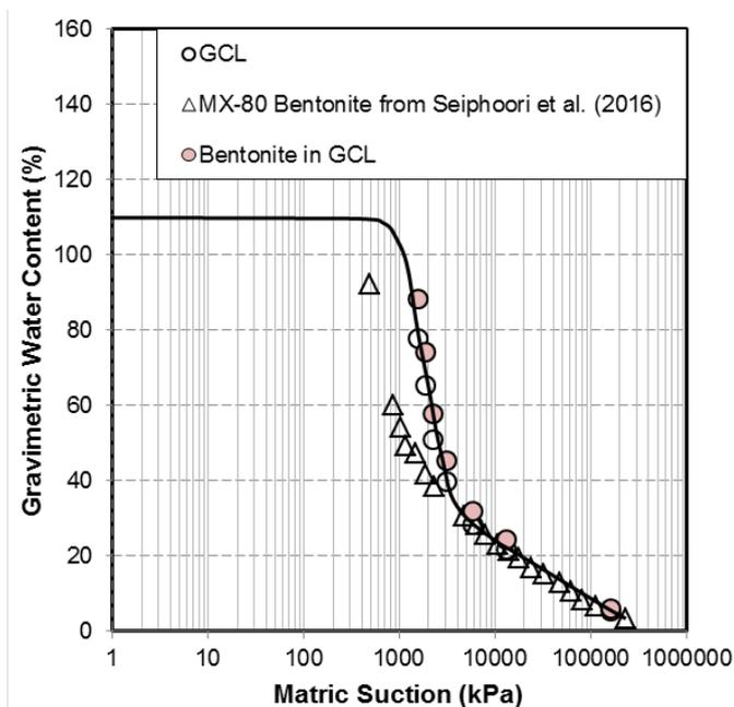
Figure 6. The WRC of bentonite in GCL.
