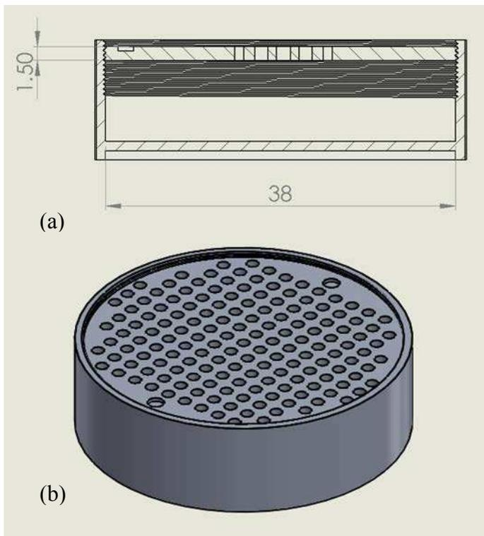
Figure 3. Schematic drawing of WP4C modified sample holder (a) cup cross-section (dimension in mm); (b) 3D view of the cup and lid (from Lu et al. 2017).
