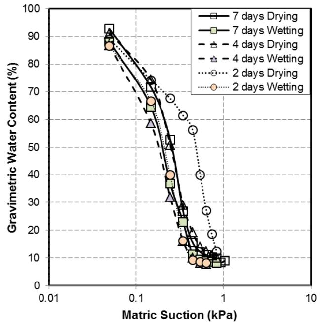
Figure 4. Capillary rise test results for initially wet and initially dry GCL strips.
