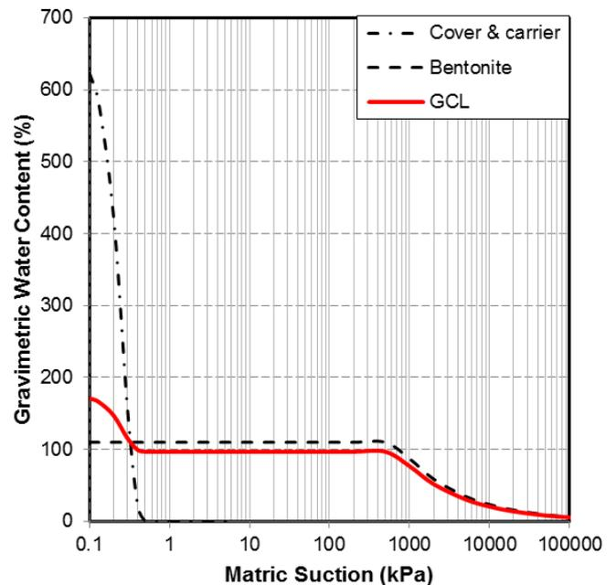
Figure 7. Deriving the WRC of GCL from superposition of the WRCs of the cover and carrier geotextiles and bentonite.
