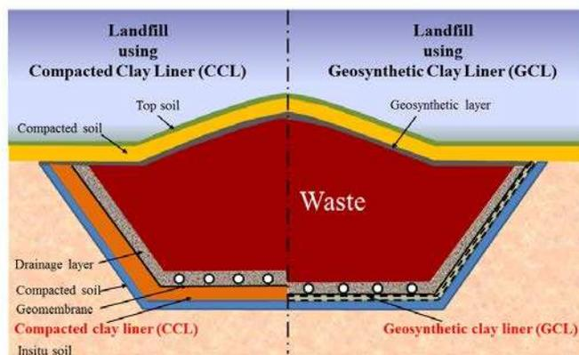
Figure 1. Schematic diagram of landfill systems using compacted clay liner and geosynthetic clay liner.
