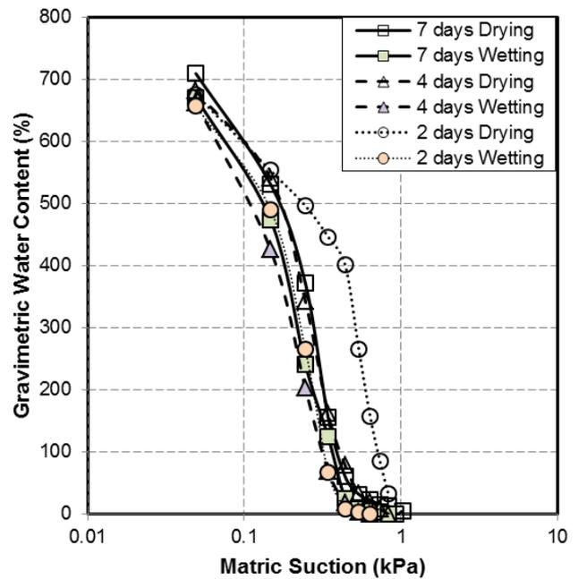
Figure 5. Water retention curves of cover and carrier geotextile layers calculated from capillary rise tests of initially wet and initially dry GCL strips.
