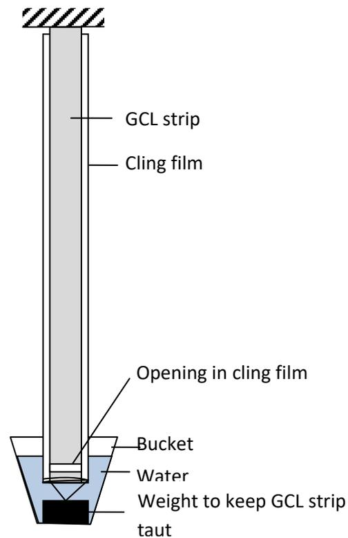
Figure 2. Schematic diagram of capillary rise test.
