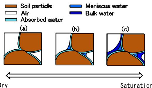
Figure 10. Pore water condition in unsaturated soil.
