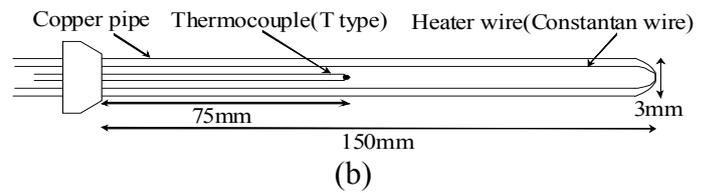
Figure 2. Thermal conductivity test device: a) Schematic of thermal conductivity test device, b) Detailed drawing of thermal probe
