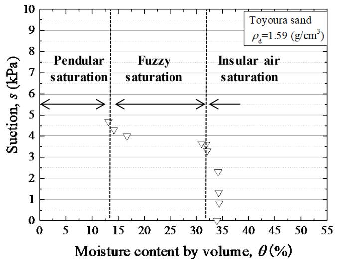
Figure 8. Soil water characteristic curve.
