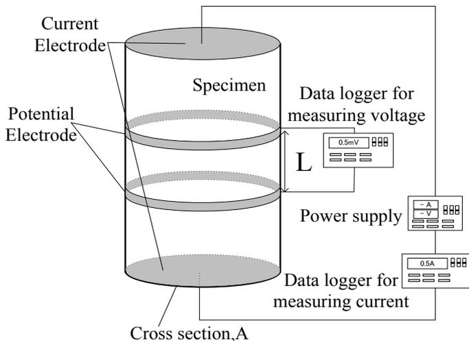
Figure 4. Electric conductivity test device.
