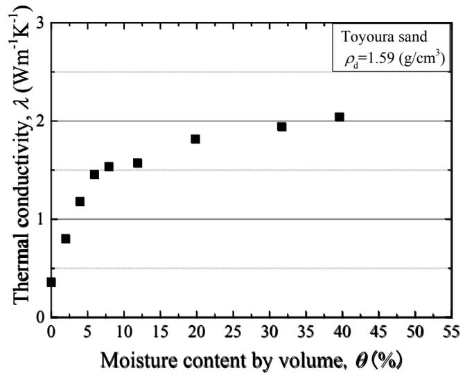
Figure 5. Thermal conductivity.
