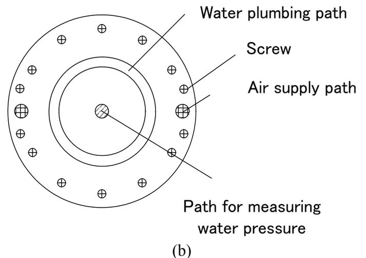
Figure 3. Permeability test apparatus: a) schematic diagram of the permeability apparatus, b) structure of cap and pedestal.
