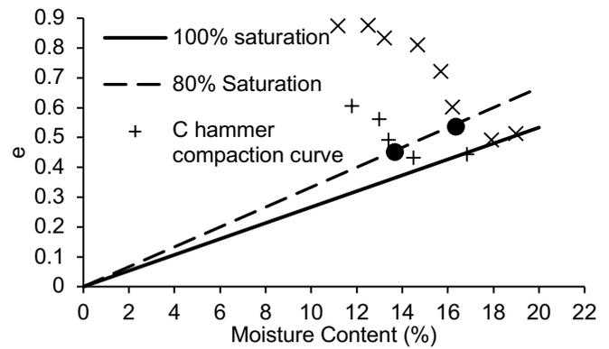
Figure 2. Typical selection method for the required densities for samples prepared using C and D compaction hammers (Kwa & Airey 2017).
