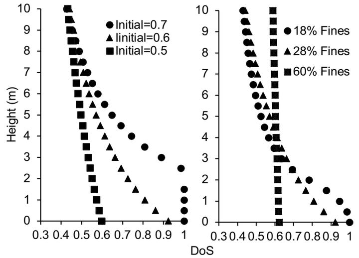
Figure 5. Variation in DoS with depth of the column with (a) increasing initial DoS for 28% fines and (b) increasing fines content at an initial DoS of 0.6.
