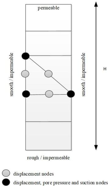
Figure 4. Schematic of one dimensional column.
