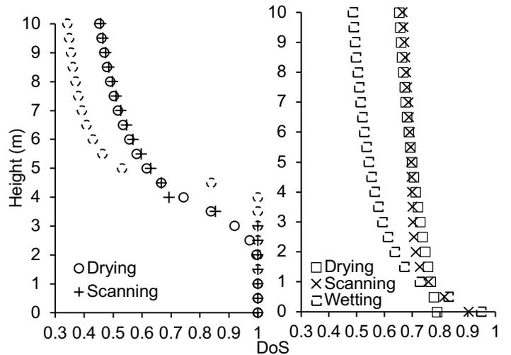
Figure 6. Variation in DoS with the depth of the column for: (a) 18% and (b) 60% fines given an initial DoS of 0.7 and initial states.
