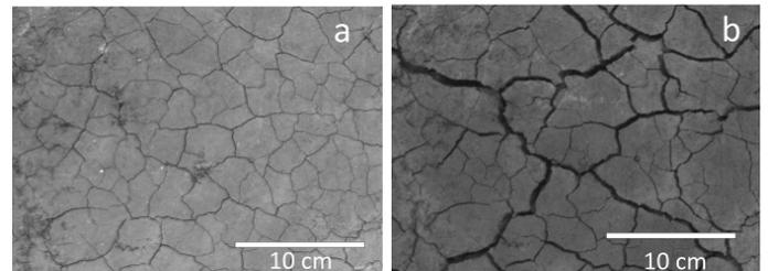
Figure 4. Crack evolution during the first drying phase: (a) surface cracks 1 and half hour of drying; (b) surface cracks at the end of drying
