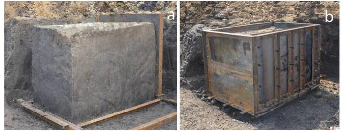
Figure 1. Soil extraction in the field: (a) trimmed soil; (b) trimmed soil in model tank
