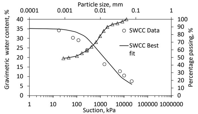
Figure 2. Soil water characteristics curve and particle distribution curve of the soil
