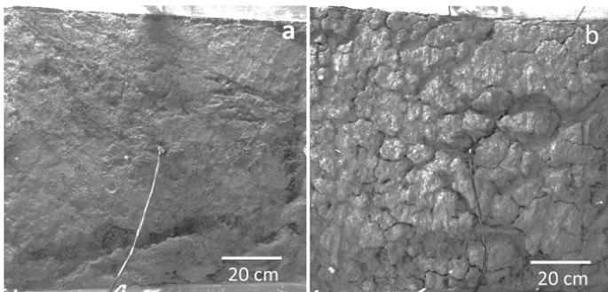
Figure 6. Soil surface morphology after wetting: (a) first cycle; (b) fifth cycle
