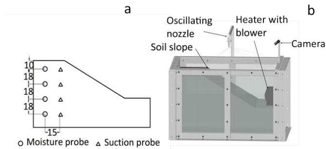
Figure 3. Instrumentation and experimental setup: (a) instrumentation; (b) experimental setup
