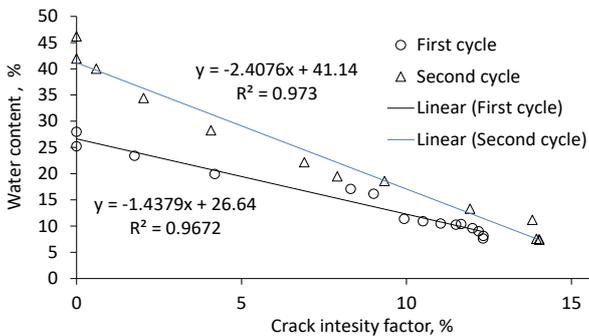
Figure 12. Variation of crack intensity factor with water content for first cycle
