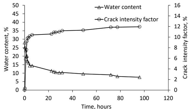
Figure 10. Change in water content and CIF with time in the first cycle
