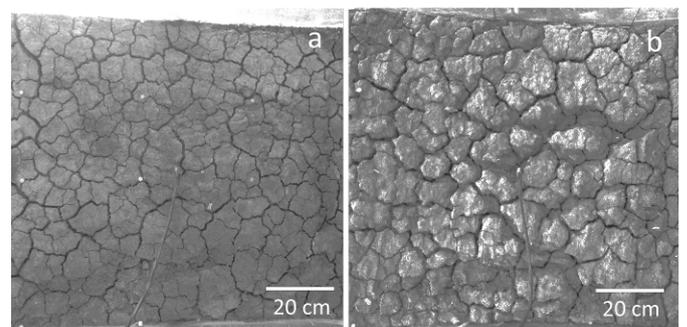
Figure 5. Evolution of surface cracks at the end of various drying cycles: (a) second cycle; (b) fifth cycle
