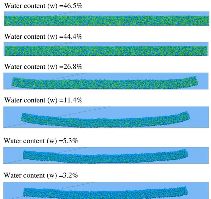
Figure 6. Shrinkage process of the simulation (blue particles are soil particles; green particles are water particles; 2D view).
