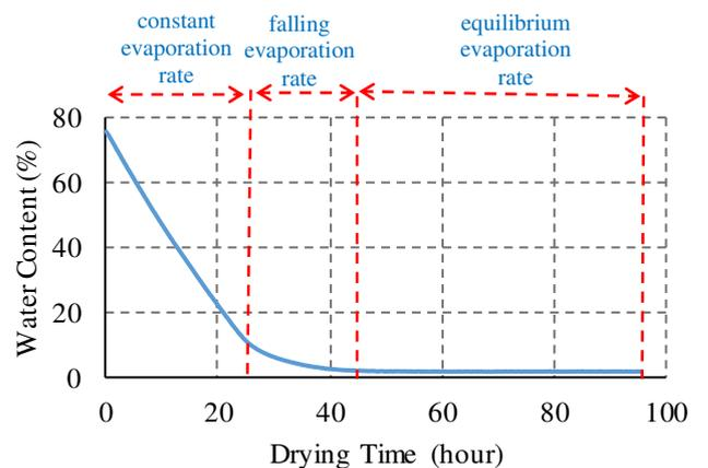
Figure 1. Water content of the specimen during drying process.
