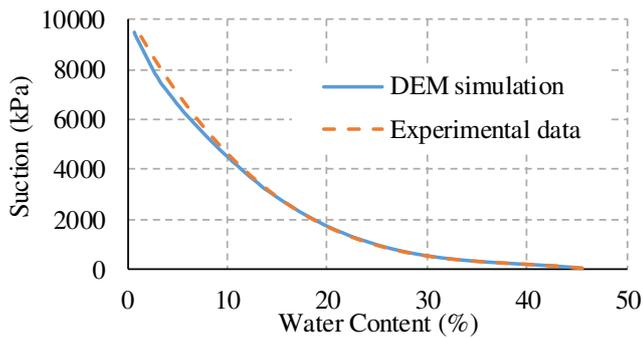
Figure 5. Soil water characteristic curves from the simulation and the experiment.
