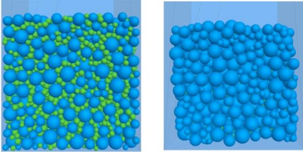
Figure 4. Model setup for calibration  $f(w)$ : before drying and after drying (blue particles are soil particles; green particles are water particles; 3D view).
