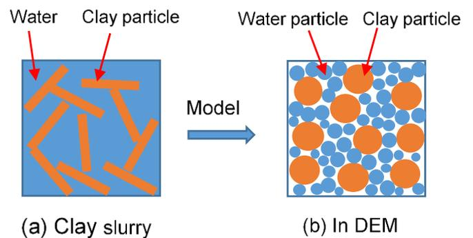
Figure 3. Water particle concept (Tran et al., 2018).
