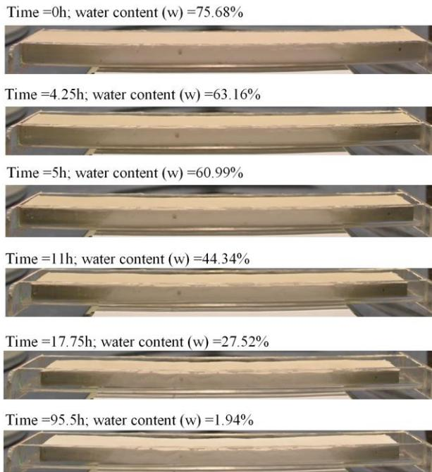
Figure 2. Shrinkage process of the kaolin clay sample.
