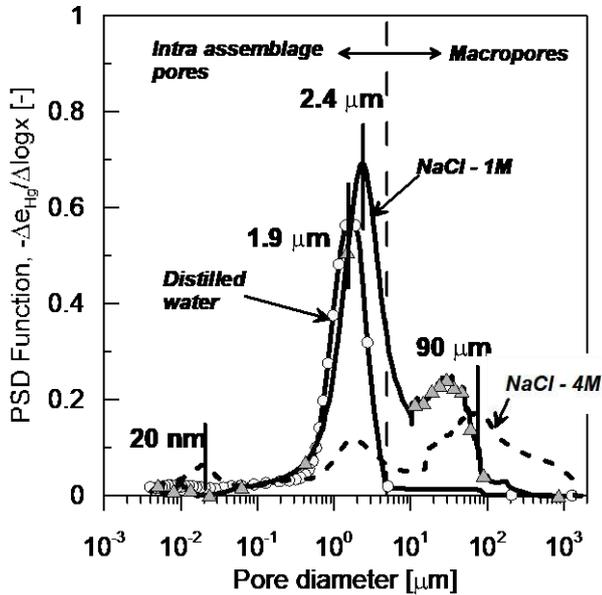
Figure 8. PSD for samples compacted to a dry density of 1.5 Mg/m<sup>3</sup> and saturated under constant volume with different types of water.
