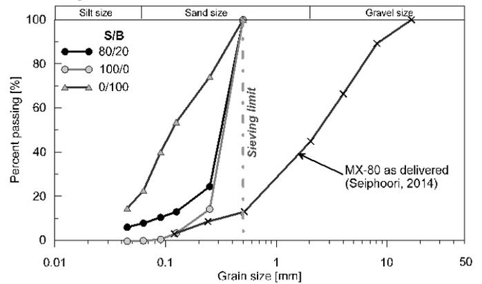
Figure 2. Apparent grain size distribution of the tested material and its two solid components. The bentonite was prepared in granular form.
