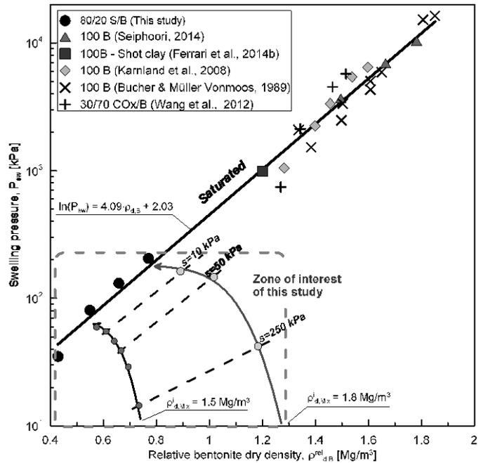
Figure 9. Swelling pressure versus relative bentonite dry density for different soil/bentonite mixtures.
