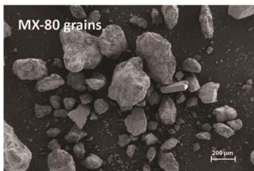
Figure 1. SEM photomicrographs of the quartz and the MX-80 bentonite grains.
