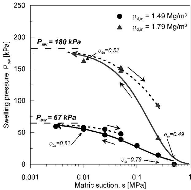
Figure 5. Evolution of the swelling pressure during a wetting process under constant volume conditions for specimen compacted to two different dry densities.
