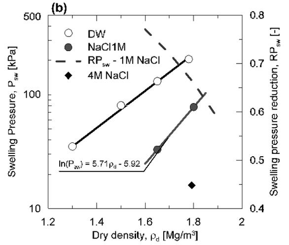
Figure 3. Swelling pressures developed with the different pore waters as a function of the dry density.
