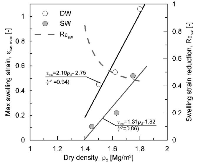
Figure 4. Results of the free swelling tests for distilled and synthetic water.
