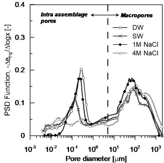
Figure 6. Pore size density functions of samples compacted to 1.5 Mg/m<sup>3</sup> and wetted with different types of water.
