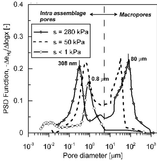
Figure 7. PSD evolution of a S/B mixture subjected to wetting process under constant volume conditions initially compacted to a dry density of 1.8 Mg/m<sup>3</sup>.
