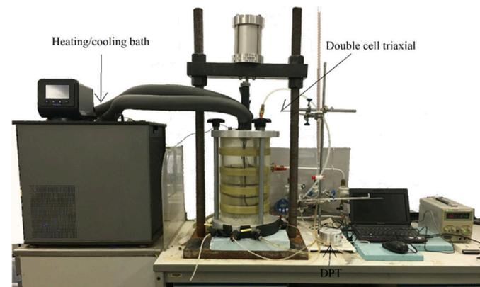
Figure 1. Photograph of the suction- and temperature-controlled double-cell triaxial apparatus
