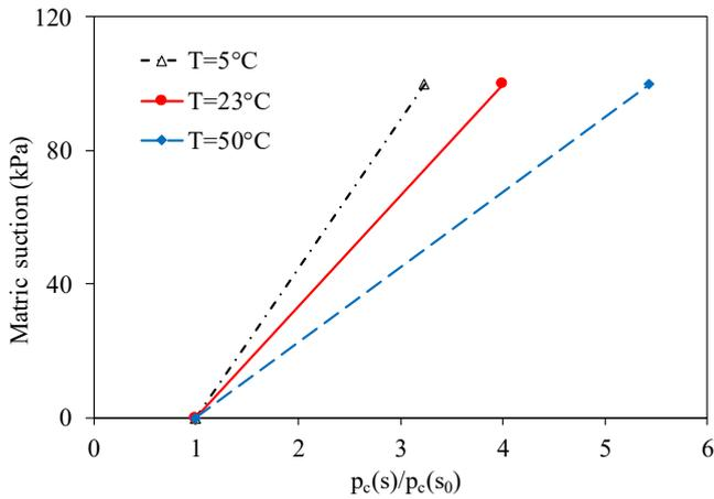
Figure 5. Wetting-induced softening of yield stress of recompacted loess at different temperatures
