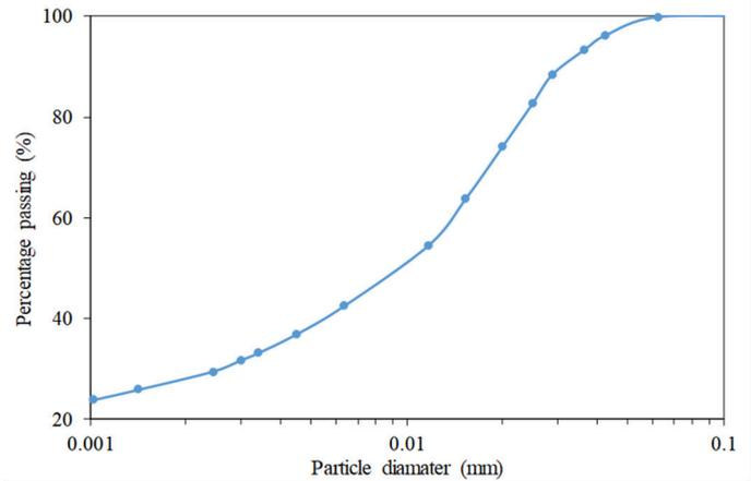
Figure 2. Particle size distribution of tested loess
