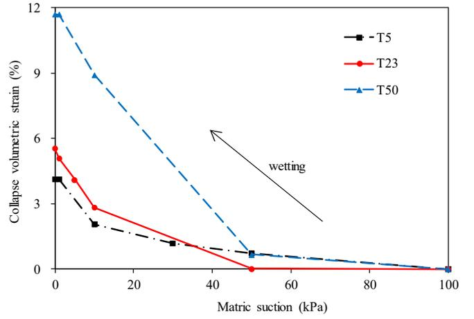
Figure 4. Wetting-induced collapse of recompacted loess during wetting from 100 to 0 kPa at different temperatures
