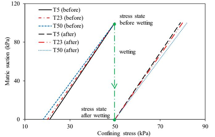
Figure 6. Thermal effects on the evolution of loading collapse curves of recompacted loess during wetting from 100 to 0 kPa
