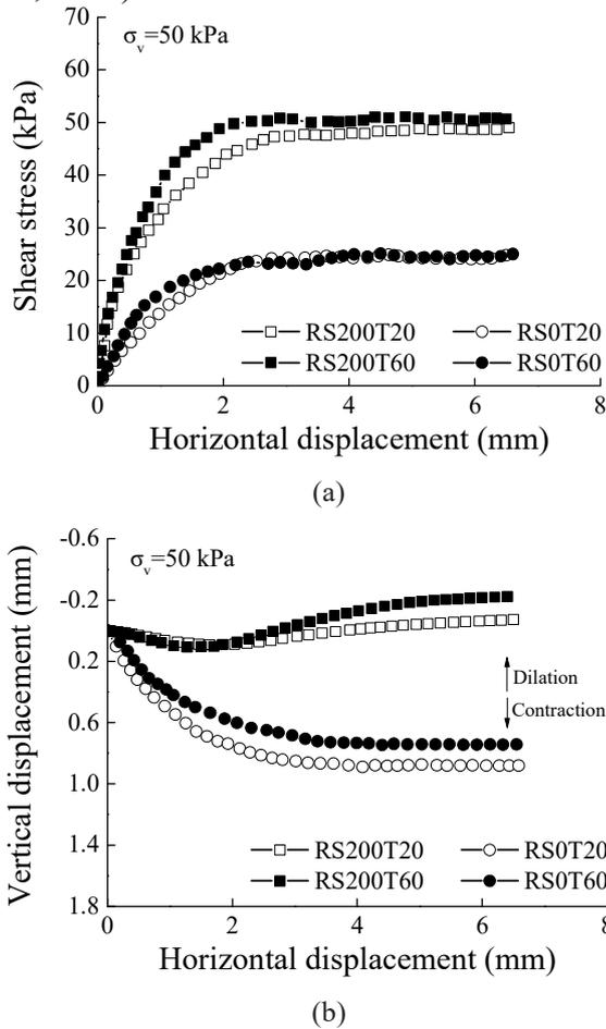
Figure 4. Thermal effects on the shear behavior of recompacted specimens: (a): stress-displacement relationship; (b): deformation behavior.
