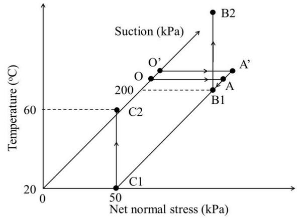
Figure 1. Thermo-hydro-mechanical test path before shearing
