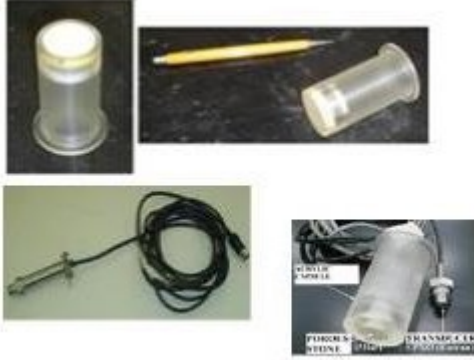
Figure 5. Acrylic body, porous stone already installed and pressure transducer used.
