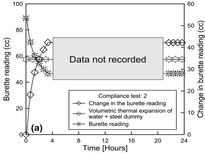
Figure 5. Test results for quantifying the volumetric thermal expansion of column.
