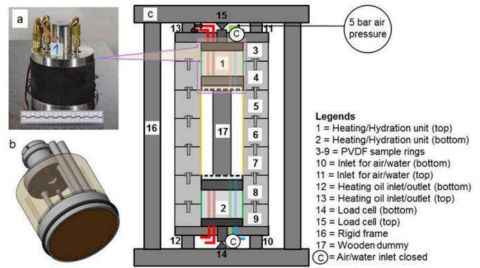
Figure 2. Schematic diagram of test setup for air/water tight construction joints, (a) top/bottom boundary control unit, (b) schematic view of top/bottom boundary control unit, and (c) test set up to validate the air/water tight joints.
