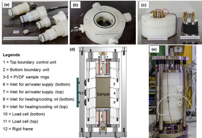
Figure 1. Technical and constructional features of newly designed column-testing device, (a) sensors, (b) PVDF sample ring with sensors, (c) top/bottom boundary control unit (d) schematic view of assembled column-testing device, and (e) pictorial view of the column-testing device.
