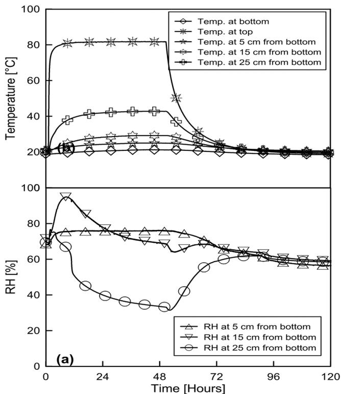
Figure 7. Test results for compliance test 3, (a) transient profile of RH values along the sample height, and (b) temperature profile at three different sections along the height of the sample.
