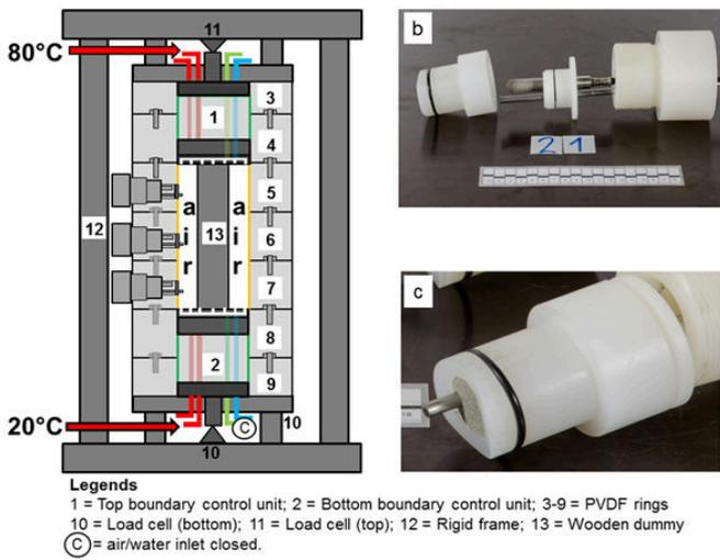
Figure 6. Schematic diagram of test setup for validating the functionality of relative humidity chambers, (a) test setup, (b) relative humidity measurement with the closed-chamber concept, and (c) closed-chamber with the extended Pt100 sensor.
