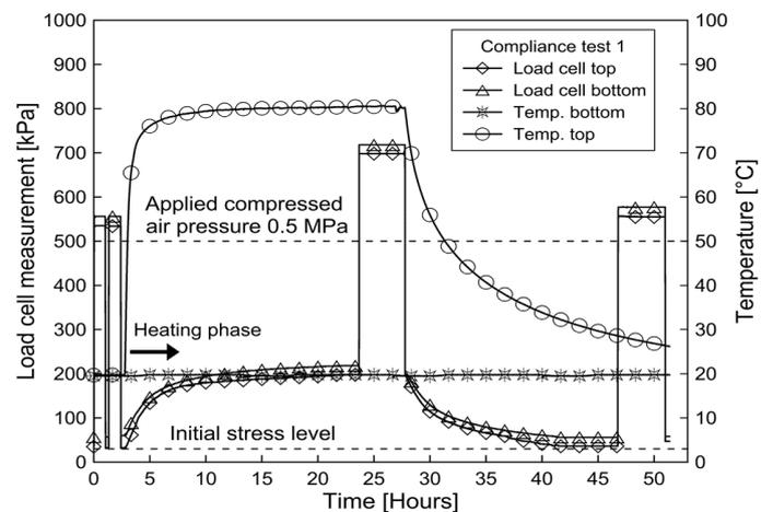
Figure 3. Test results for air/water tight joints under 0.5 MPa compressed air pressure.
