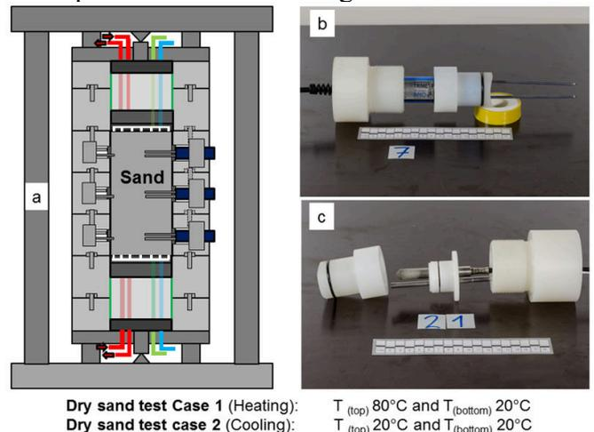
Figure 8. Schematic diagram of test setup with dry sand (a) test setup with RH chambers and TDRs, (b) installation of TDR with PVDF sensors adapter, and (c) RH chamber.
