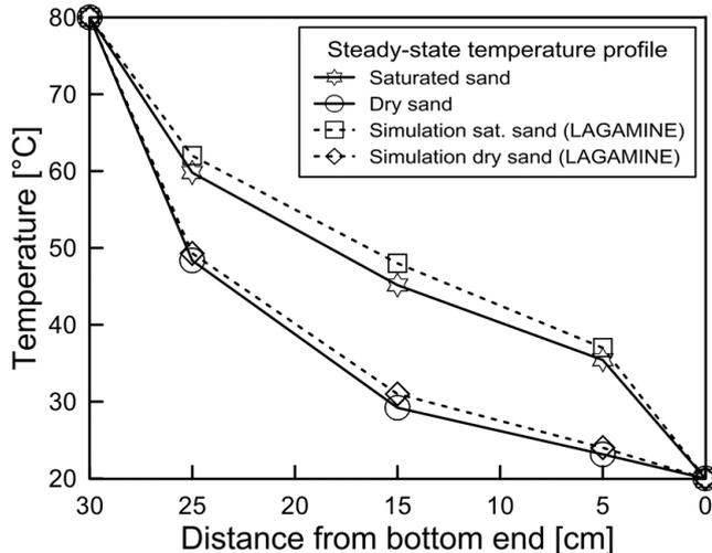
Figure 10. Test results for one-dimensional heat flow condition with dry and fully saturated sand.
