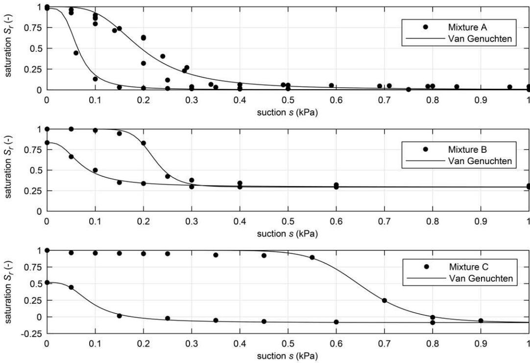
Figure 5. Retention behaviour of the three investigated mixtures A, B, and C obtained from drainage and imbibition experiments. Fitted curves using the model by van Genuchten (1980) are also depicted.
