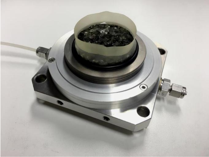
Figure 4. Assembled specimen base pedestal equipped with a fully saturated specimen made of mixture A.
