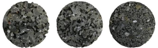
Figure 2. Top view on specimens of drilling cores with a diameter of 50 mm. Mixture A (left), mixture B (middle), mixture C (right).
