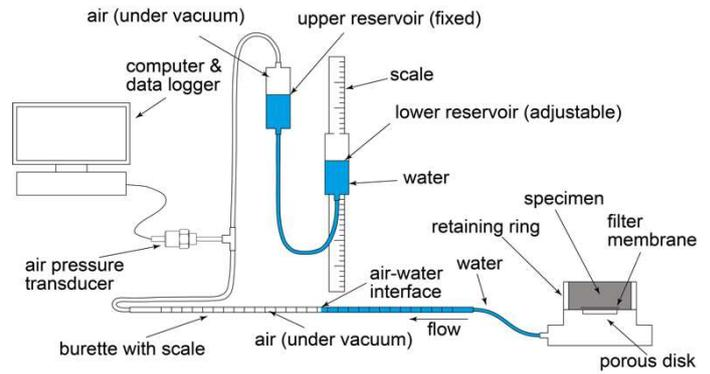
Figure 3. Modified hanging water column apparatus following ASTM D6836-16
