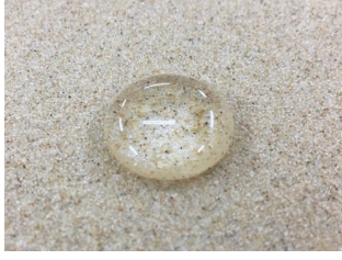
Figure 1. A water droplet on water repellent Toyoura sand.
