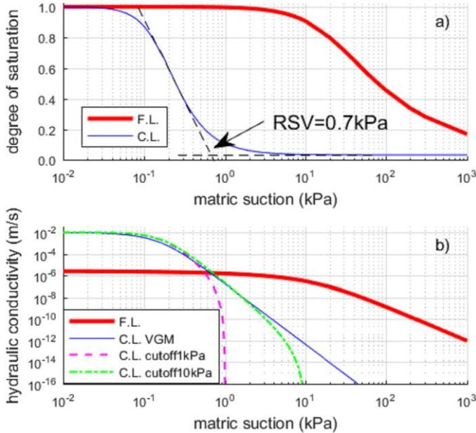
Figure 2. Hydraulic properties of the materials: a) soil water retention curves and b) hydraulic conductivity curves
