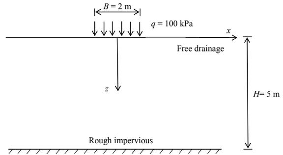
Figure 5. Boundary conditions for 2D plane strain consolidation of unsaturated soil.
