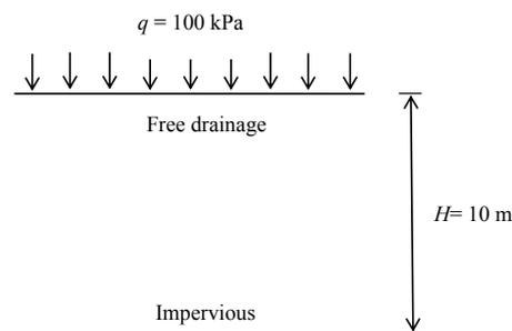
Figure 2. Boundary conditions for 1D consolidation.
