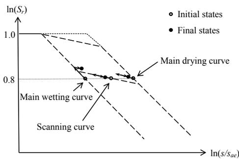
Figure 4. For a certain initial degree of saturation, illustration of how the hydraulic states move on a normalized SWCC during consolidation for different initial hydraulic state locations.
