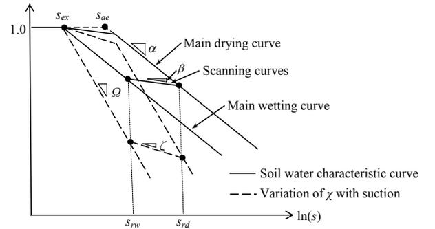
Figure 1. The soil-water characteristic curve with hydraulic hysteresis and the relationship between  $\chi$  and  $s$ .
