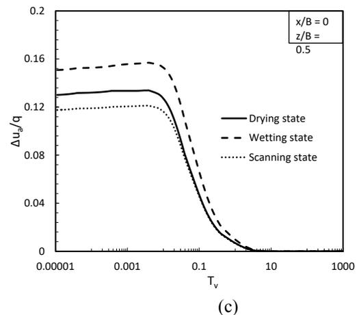
Figure 6. Numerical simulation of 2D plane strain consolidation of unsaturated soil with different initial locations of hydraulic states: (a) normalized settlement; (b) normalized excess water pressure; (c) normalized excess air pressure; versus dimensionless time factor.
