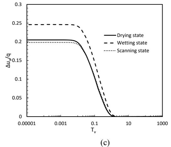
Figure 3. Numerical simulation of 1D consolidation of unsaturated soil with different initial locations of hydraulic states: (a) normalized settlement; (b) normalized excess water pressure; (c) normalized excess air pressure; versus dimensionless time factor.
