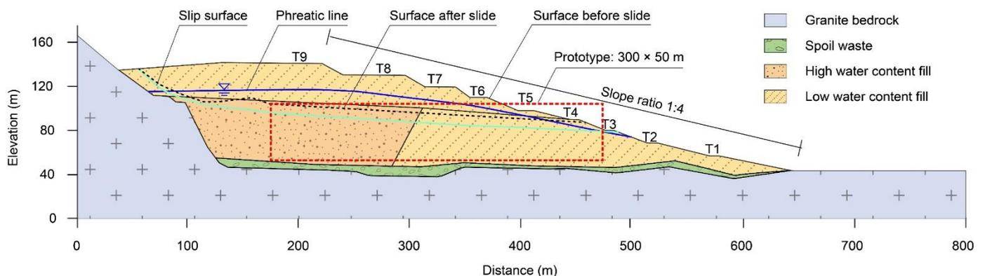
Figure 1. Geotechnical profile before and after the landslide.
