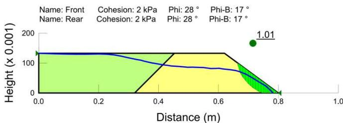
Figure 6. Back calculations by using 2-D numerical model with LEM.
