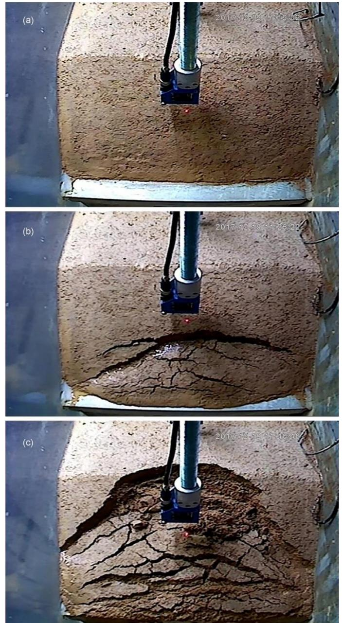
Figure 4. Failure of model slope: (a) 0 g; (b) 18 g; (c) 20 g.
