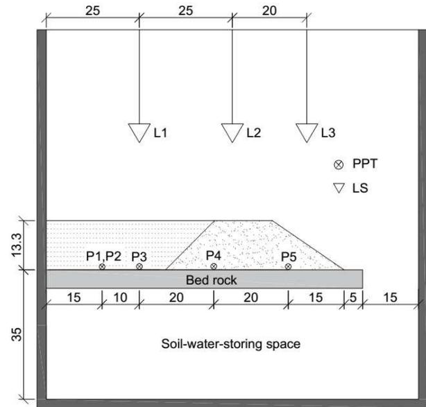
Figure 2. Test setup of the slope model (unit: cm).
