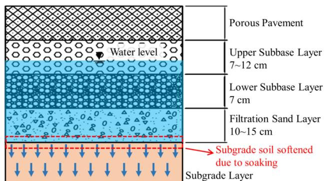
Figure 1. Profile of a road base with porous pavement (PCC 2007)
