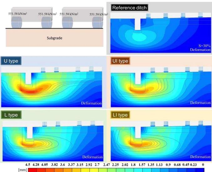
Figure 9. Spatial distribution of deformation in subgrade soil under truck loading (tire pressure 80 psi).
