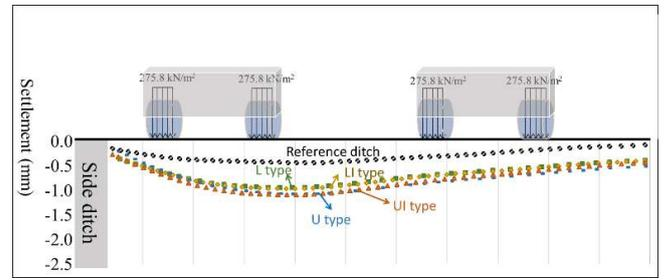
Figure 10. Settlement troughs of car loading (tire pressure 40 psi).
