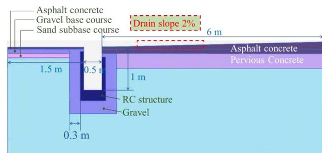
Figure 4. Model configuration for the numerical analysis of U type side ditch.
