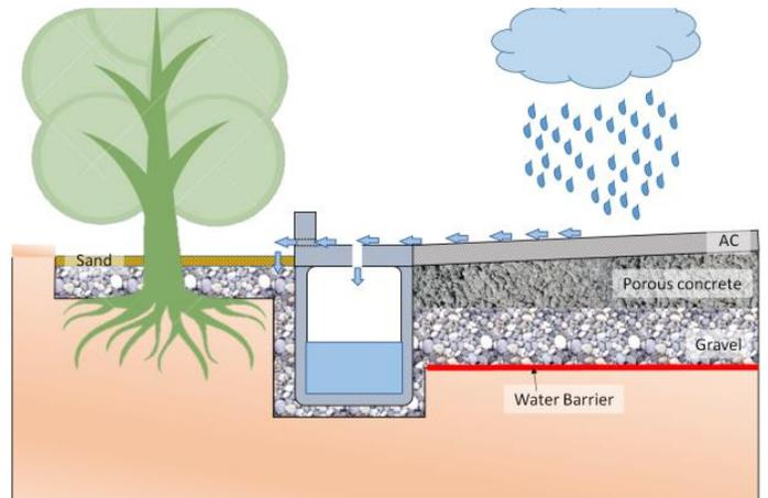
Figure 13. Details of UI type side ditch and gravel backfill.
