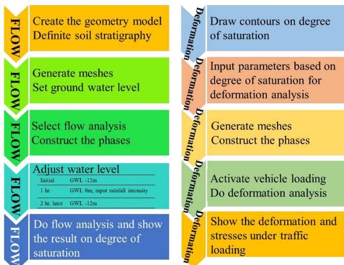
Figure 5. Procedures of the flow and deformation analyses.
