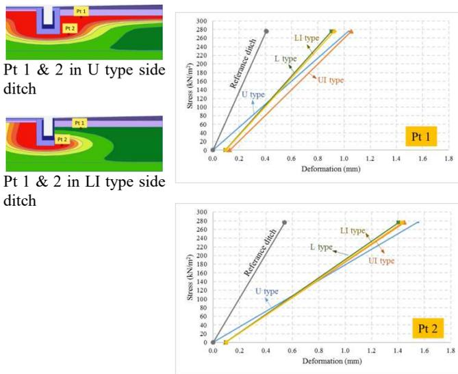
Figure 12. Stress-deformation of mark points 1 and 2 for different side ditch configurations.
