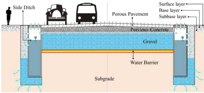
Figure 2. Integrated road base and side ditch system with separated water preservation layer and porous side ditch (Guo 2017).
