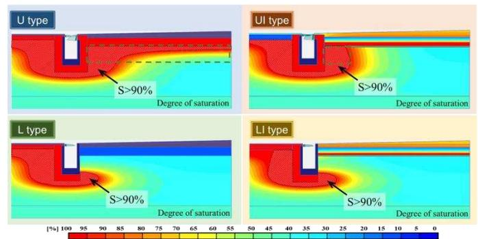
Figure 7. Spatial distribution of degree of saturation for four types of side ditch studied in the flow analysis.
