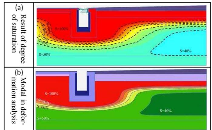
Figure 8. Converting model parameters from flow analysis to deformation analysis.
