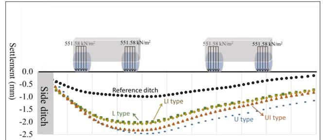
Figure 11. Settlement troughs of car loading (tire pressure 40 psi).
