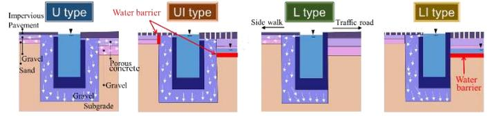
Figure 3. Four types of side ditch configuration studied in this research.
