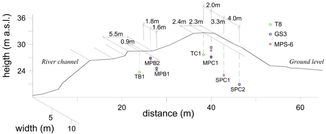
Figure 4. Layout of the monitoring points.
