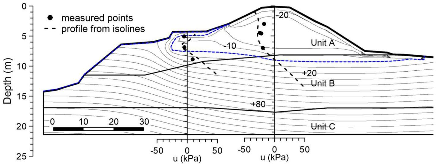
Figure 6. Comparison of pore pressure profile at 07/02/2017 from monitoring data (solid circles) and numerical model (isolines).
