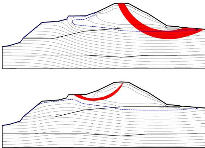
Figure 7. Riverbank safety map for outer slopes and inner slopes critical surfaces (07/02/2017).
