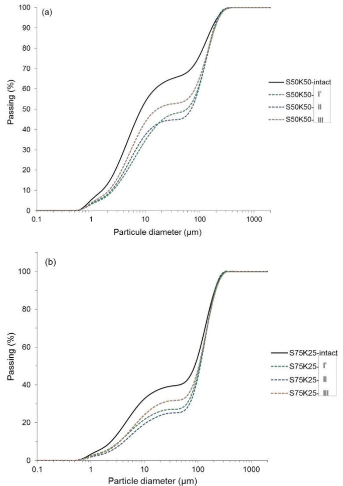
Figure 6. Influence of traffic cycles on grain size distribution of soil (a) S50K50, (b) S75K25.
