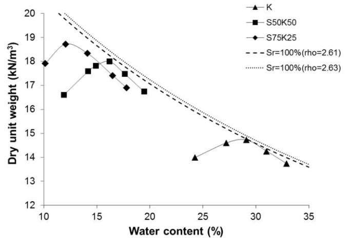
Figure 2. Normal Proctor compaction curves of tested soils.
