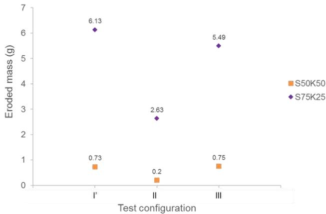
Figure 5. Influence of traffic cycles on compacted soil surface degradation.
