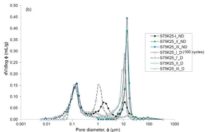
Figure 8. Influence of traffic cycles on pore size distribution of soil not degraded (ND) and degraded (D): (a) S50K50; (b) S75K25.
