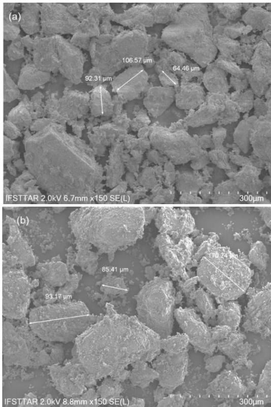
Figure 7. SEM observations of eroded soil at the surface specimens compacted at configuration 'III' (a) S50K50, (b) S75K25.
