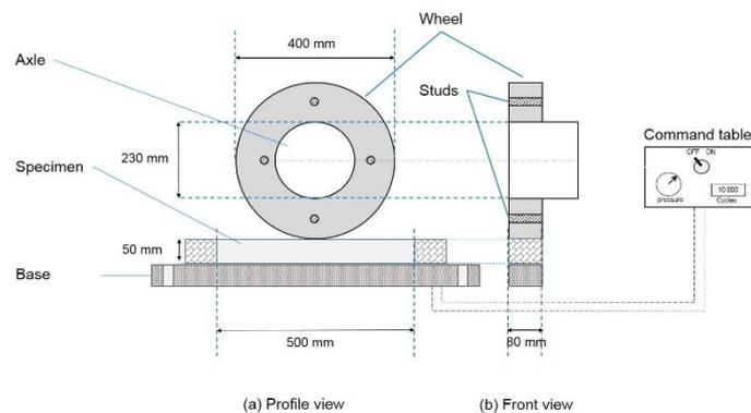
Figure 3. Scheme of Laboratory Traffic Simulator (LTS).
