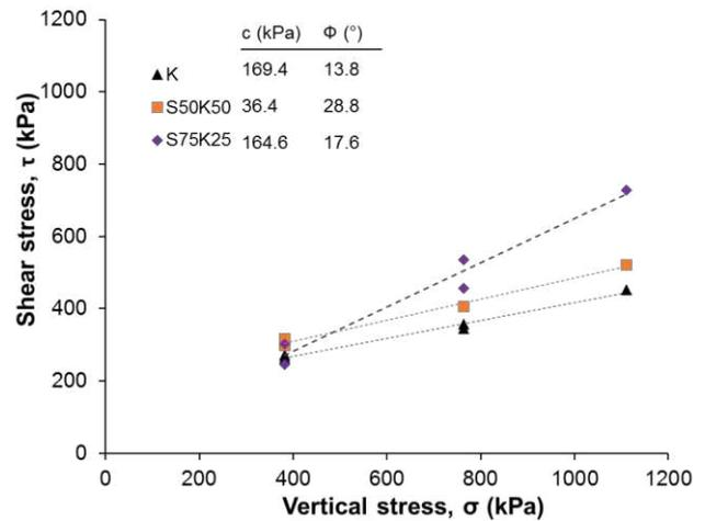
Figure 4. Results of direct shear tests of studied soils.
