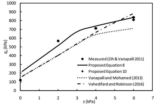
Figure 3. Comparison between measured and predicted bearing capacities of square footing on coarse sand (Oh & Vanapalli 2011).
