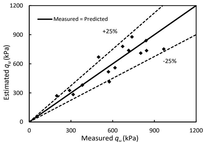
Figure 6. Comparison between measured and predicted bearing capacities based on the proposed equations.
