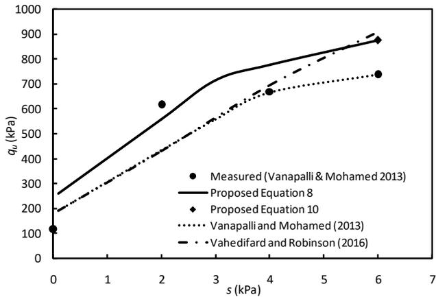
Figure 5. Comparison between measured and predicted bearing capacities of square plate on coarse sand (Vanapalli & Mohamed 2013).
