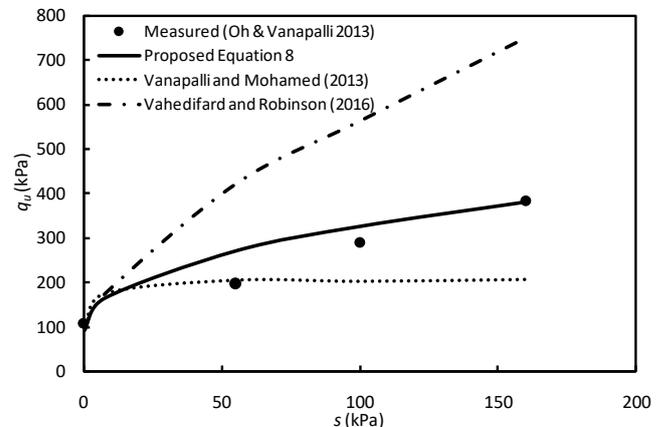
Figure 4. Comparison between measured and predicted bearing capacities of square footing on fine grained soil (Oh & Vanapalli 2013).
