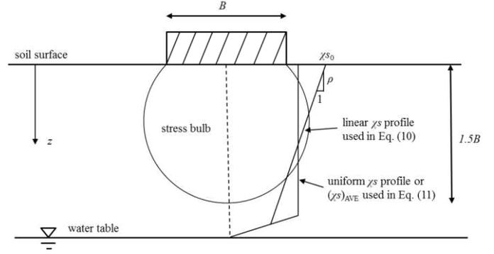
Figure 1. Typical uniform and linear  $\chi s$  profiles in unsaturated soil under a footing.
