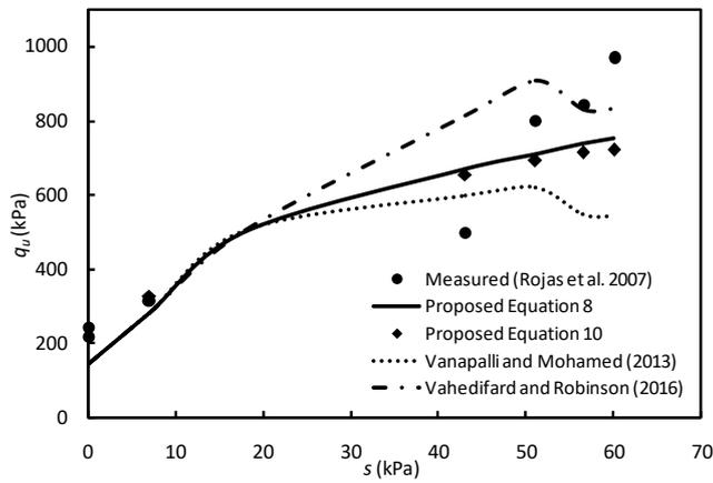
Figure 2. Comparison between measured and predicted bearing capacities of plate on lean clay (Rojas et al. 2007).
