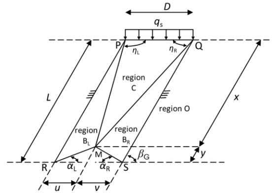
a. The geometry of a hang-up in a plane inclined ore pass.
