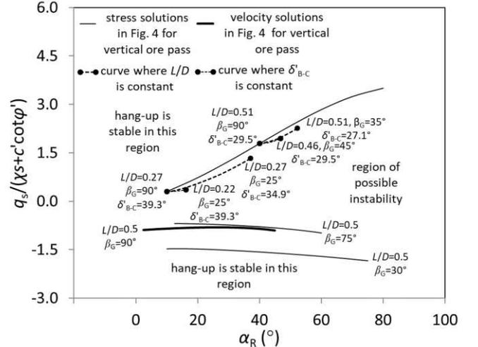
b. Discontinuous stress solutions and discontinuous velocity solutions for when  $\varphi' = 40^\circ$ .
