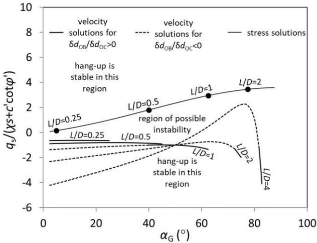
Figure 4. Comparison of discontinuous stress and velocity solutions for a bursting failure mechanism in plane vertical ore pass for when  $\varphi' = 40^\circ$ .
