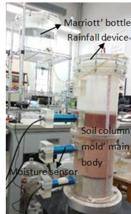
Figure 1. Schematic setup of soil column test.
