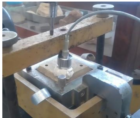
Figure 2. Direct Shear Apparatus incorporated with a tensiometer.
