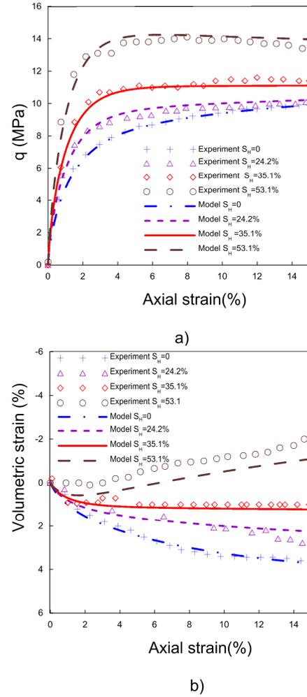
Figure 2: Comparisons between model and experimental results for synthetic samples of HBS prepared at different  $S_h$ : a) stress-strain behavior; and b) volumetric strain versus axial strain; (experimental data from (Hyodo et al., 2014)).
