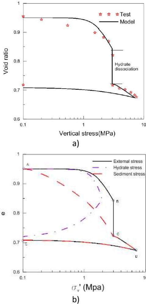
Figure 3: Behavior during dissociation of natural GHBS specimens under oedometric conditions: (experimental data from (Santamarina et al., 2015)).
