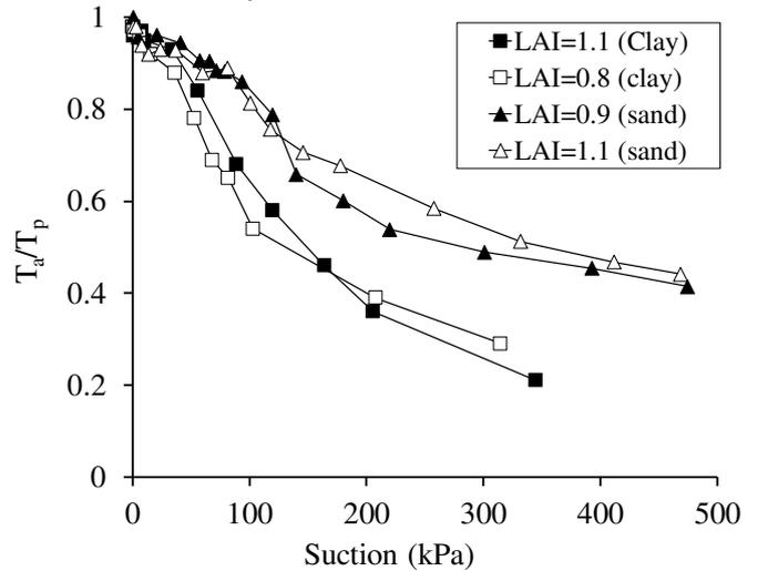
Figure 4. Effects of soil type on transpiration reduction function
