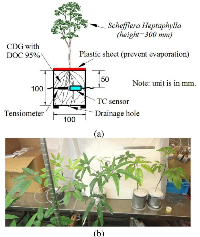
Figure 1. (a) Schematic diagram for test setup and instrumentations and (b) Overview of test setup in plant room
