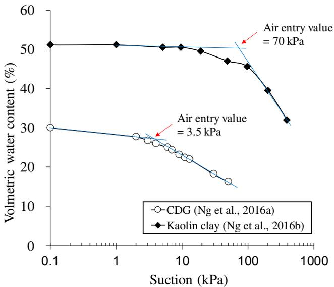
Figure 2 Soil water retention curves (SWRCs) of tested soils
