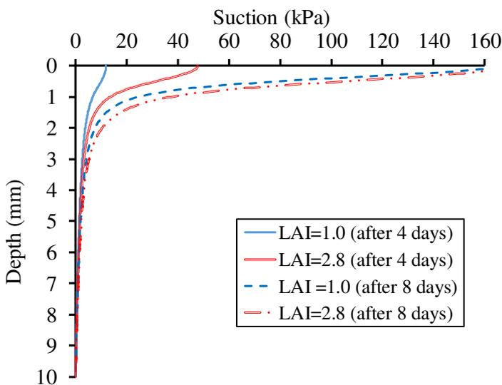
Figure 5. Effects of LAI on induced soil suction
