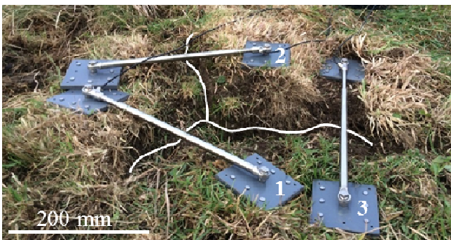
Figure 4. Transducer configuration at monitored crack site.
