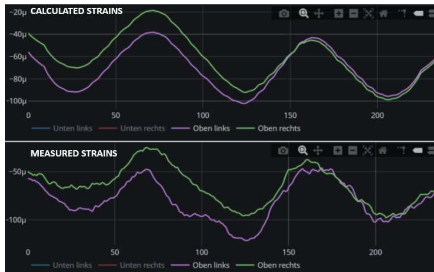
Figure 8: Comparison of calculated and measured strains: the difference is less than 5%.
